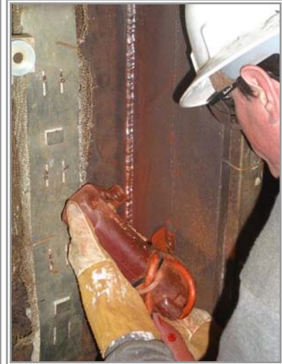
Typical MT of PJP with Model B-100 Parker Probe
