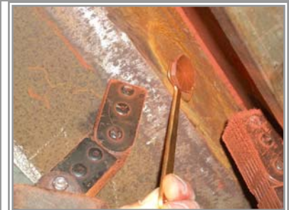
Verifying MT Sensitivity of B-100 Parker Probe with Pie Guage
