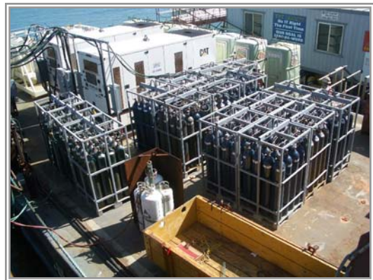
Welding Gas Mixture Storage
