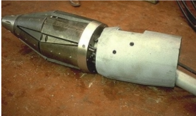
Figure 18. Standard Pipe Bursting Head. (18)
