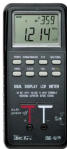
Figure 32. Photo. Handheld instrument for performing AC impedance measurements.
