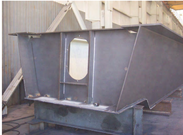
Figure 12.3 Solid Plate Interior Support Diaphragm with Access Hole
