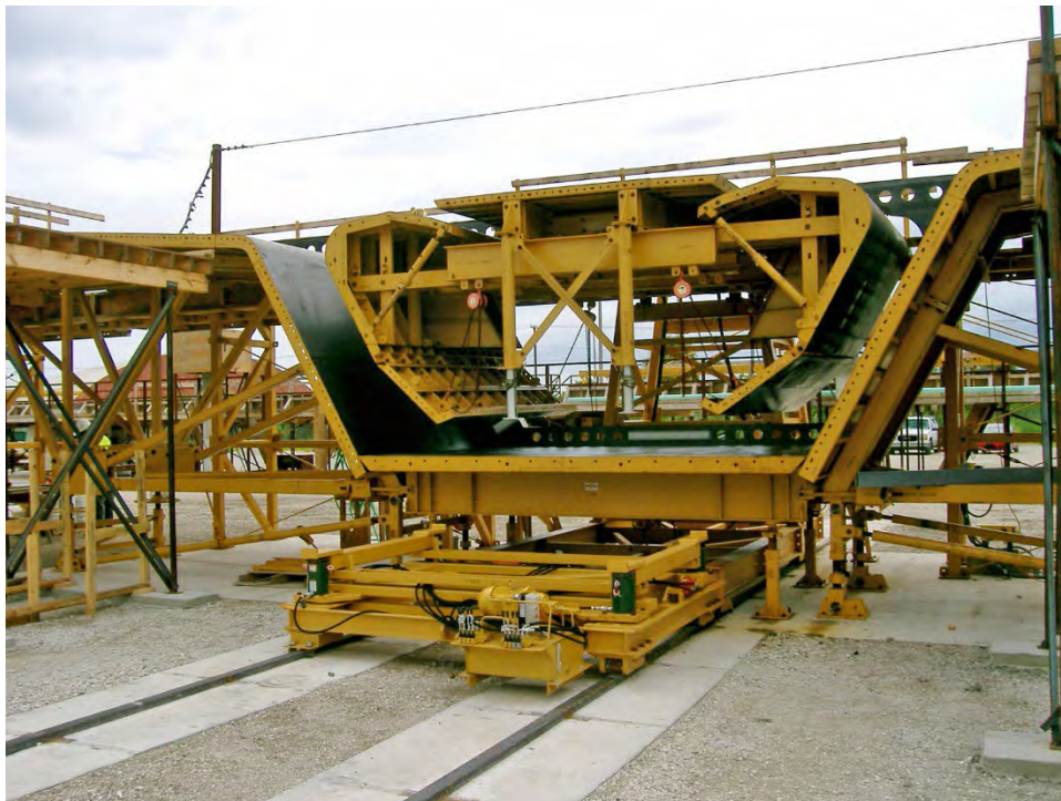
Figure 8.7 Casting Machine for Short-Line Segment Casting
