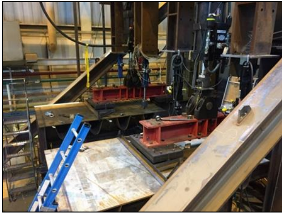
Figure 2. Slit RFB Connection test specimen
