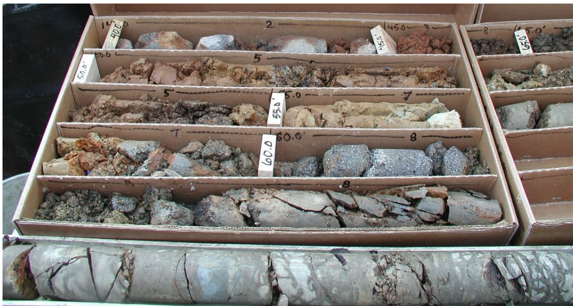
Figure 5-1 Rock core showing wide range in rock mass characteristics – photo by authors.
