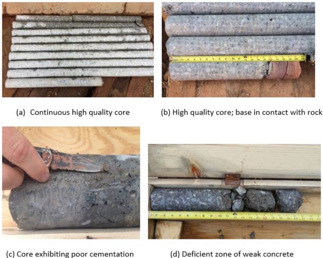
Figure 5-3 Examples of Features Observed in Concrete Core – photos by the authors.
