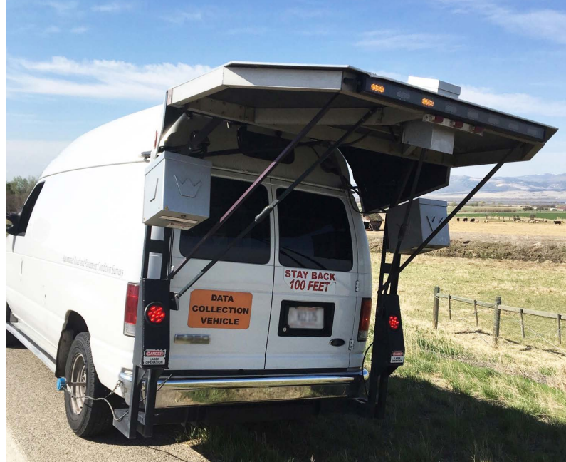
Ensuring data quality will help States address Federal requirements for national performance measures. Here, the Montana Department of Transportation prepares to collect pavement surface distress measurements (such as rutting, cracking, and faulting). Source: FHWA.
