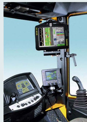
Intelligent compaction equipment provides real-time feedback to the roller operator measuring the number of roller passes on each section of mat. Source: NHI.
