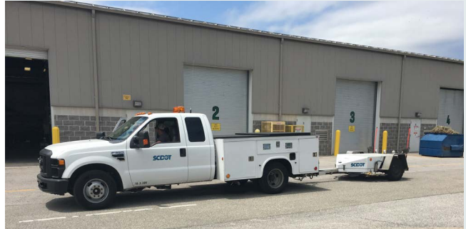
A locked-wheel skid trailer, such as this one owned by the South Carolina Department of Transportation, is currently the most commonly used equipment for friction measurement in the United States. Source: FHWA.
