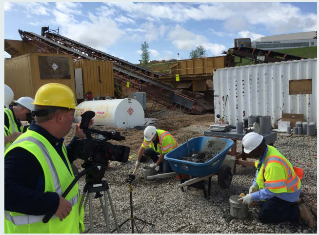
The production crew collects video footage of workers preparing samples for Super Air Meter testing. Photo: ©Jagan Gudimetta, ATI, Inc.
