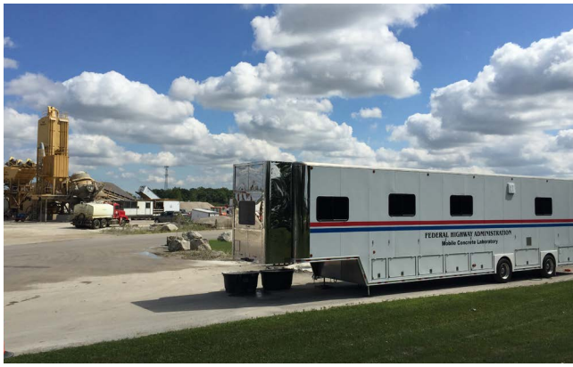
The MCTC is set up on a concrete production facility. A concrete batch tower and mixing plant are visible behind the trailer. Source: FHWA.
