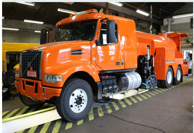
Continuous friction measurement equipment, as shown here, provides a much higher spatial coverage and reduces the chances of missing localized areas with friction deficiencies. Source: FHWA.
