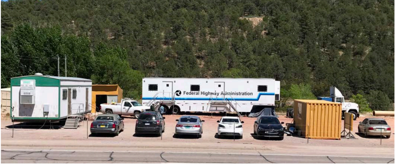
FHWA uses the Mobile Asphalt Testing Trailer, pictured here staged adjacent to a highway resurfacing project near Albuquerque, NM, to introduce innovations, new technology, and test methods to pavement engineers across the United States. Source: APTech.
