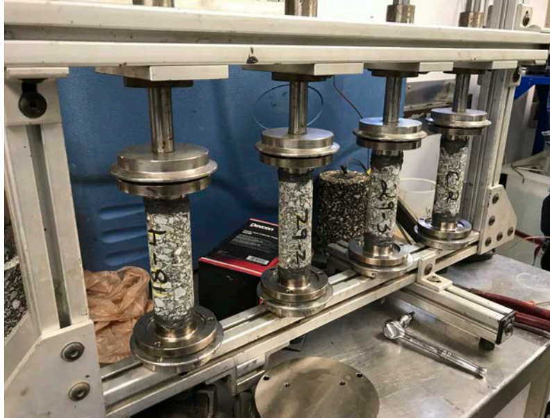
Small-diameter specimens for the Asphalt Mixture Performance Tester are affixed in a jig awaiting attachment of deformation sensors. Source: APTech.
