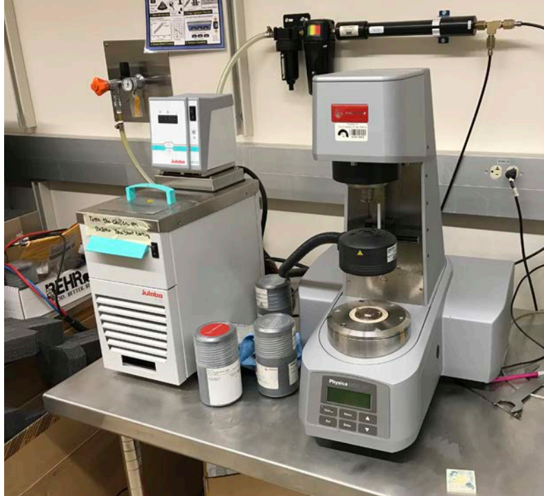
The dynamic shear rheometer (DSR) tests the viscous and elastic behavior of asphalt binders and is one of the lab tests that required different tools and sample geometry modification to accurately evaluate GTR materials and other modifiers in the binder. Source: APTech.
