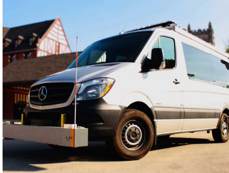
This van is equipped with high-speed data collection equipment. Source: APTech.
