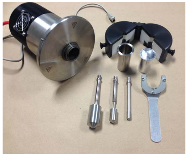
Closeup of GTR testing components of the DSR. Rather than testing a flat, thin, circular specimen of asphalt binder, the modified DSR test tools, called concentric cylinders, require that a sample of GTR modified asphalt binder be poured into a small metal cup (outer cylinder) and then tested in shear using one of three different bobs (inner cylinders). Source: FHWA.
