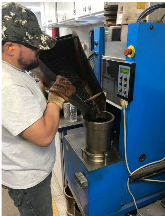
To prepare for performance testing, a technician loads asphalt mixture into a compaction mold. The mixture is compacted, and then four small specimens are removed from the sample using a core barrel and drill press. Source: FHWA.
