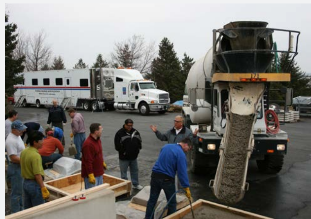
FHWA's Mobile Concrete Trailer is being used to provide hands-on training on PEM test procedures. Source: Jagan Gudimettla/FHWA Mobile Concrete Trailer.
