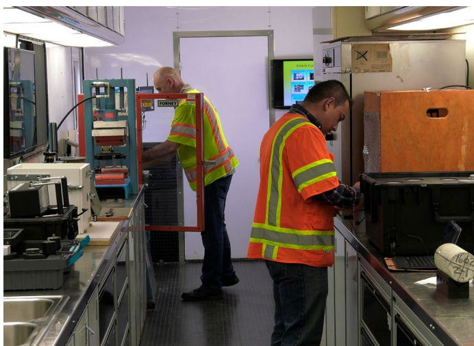
MCTC staff performing testing inside the mobile concrete laboratory. Source: FHWA
