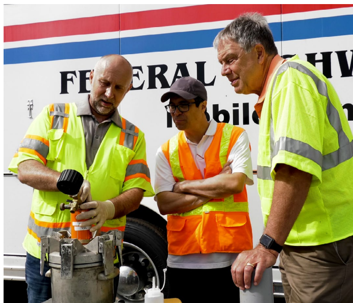
MCTC staff demonstrating durability testing using the Super Air Meter. Source: FHWA
