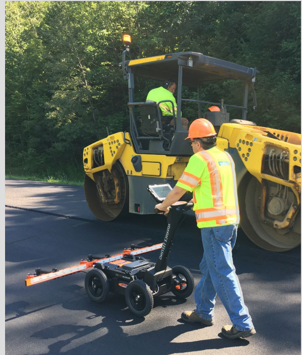
Dielectric profiling system for measuring asphalt pavement density. Source: Rob Sommerfeldt, GSSI
