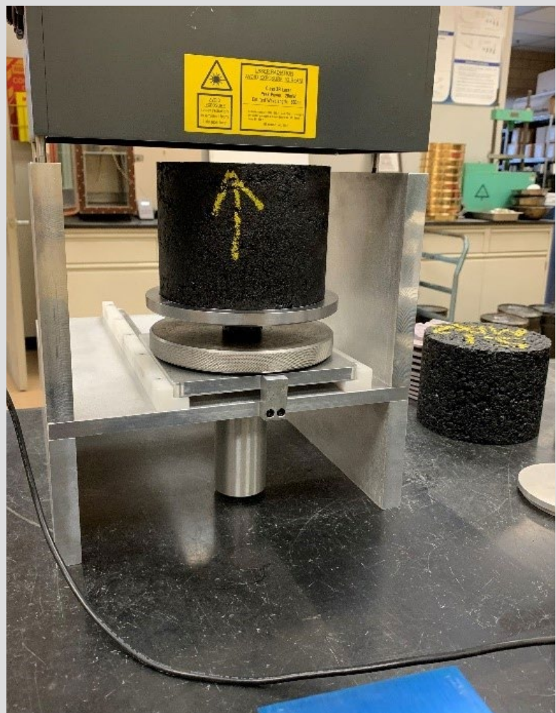
Measuring macrotexture of laboratory-prepared gyratory specimen using rapid laser texture scanner. Source: FHWA
