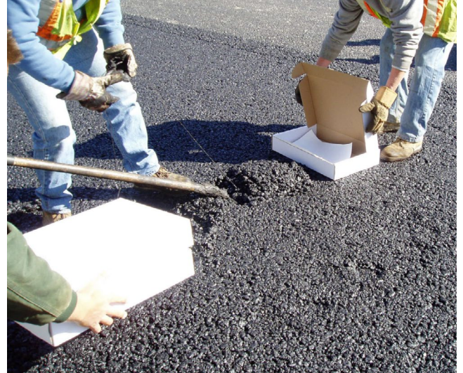
Sampling behind paver to obtain loose sample of asphalt mixture. Source: FHWA
