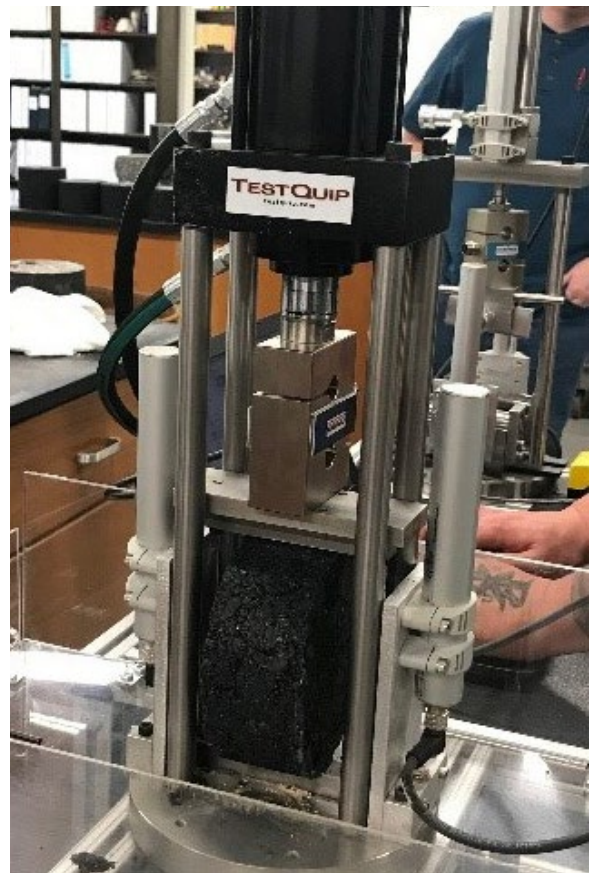
Indirect Tensile Asphalt Cracking Test Source: FHWA
