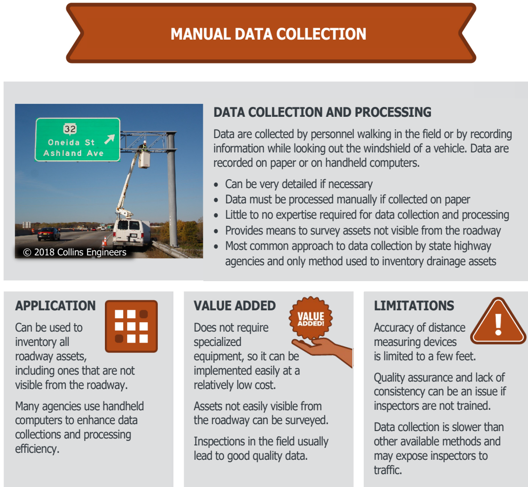
Figure 24. Graphic. Characteristics associated with manual data collection techniques (adapted from Zimmerman and Manda 2015 with permission from National Academy of Sciences, courtesy of the National Academies Press, Washington, DC).
