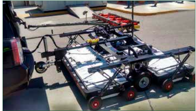
Figure 2: IDS Stream-EM (with GPS) MCGPR towed antenna array
