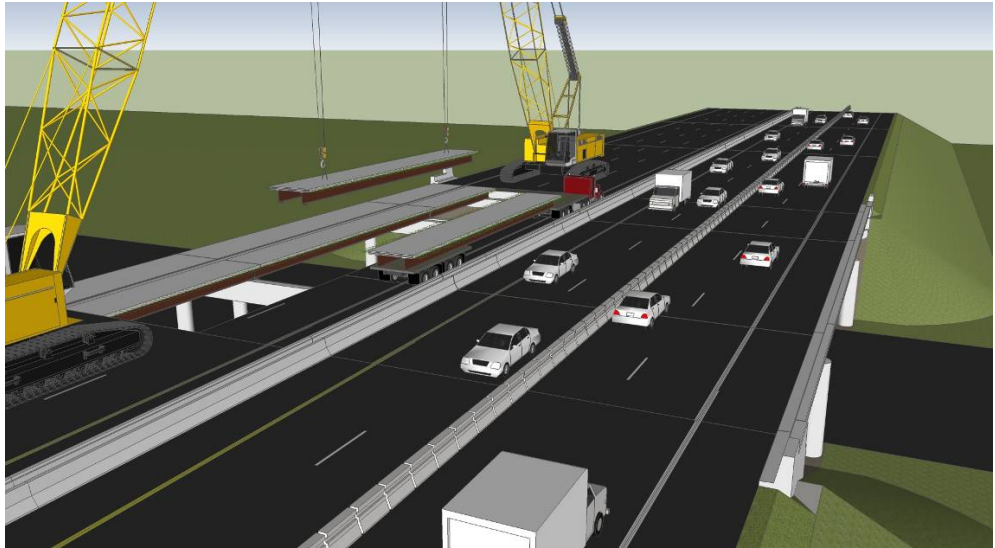
Figure 2.3.1-4 I-93 Superstructure Replacement Concept
