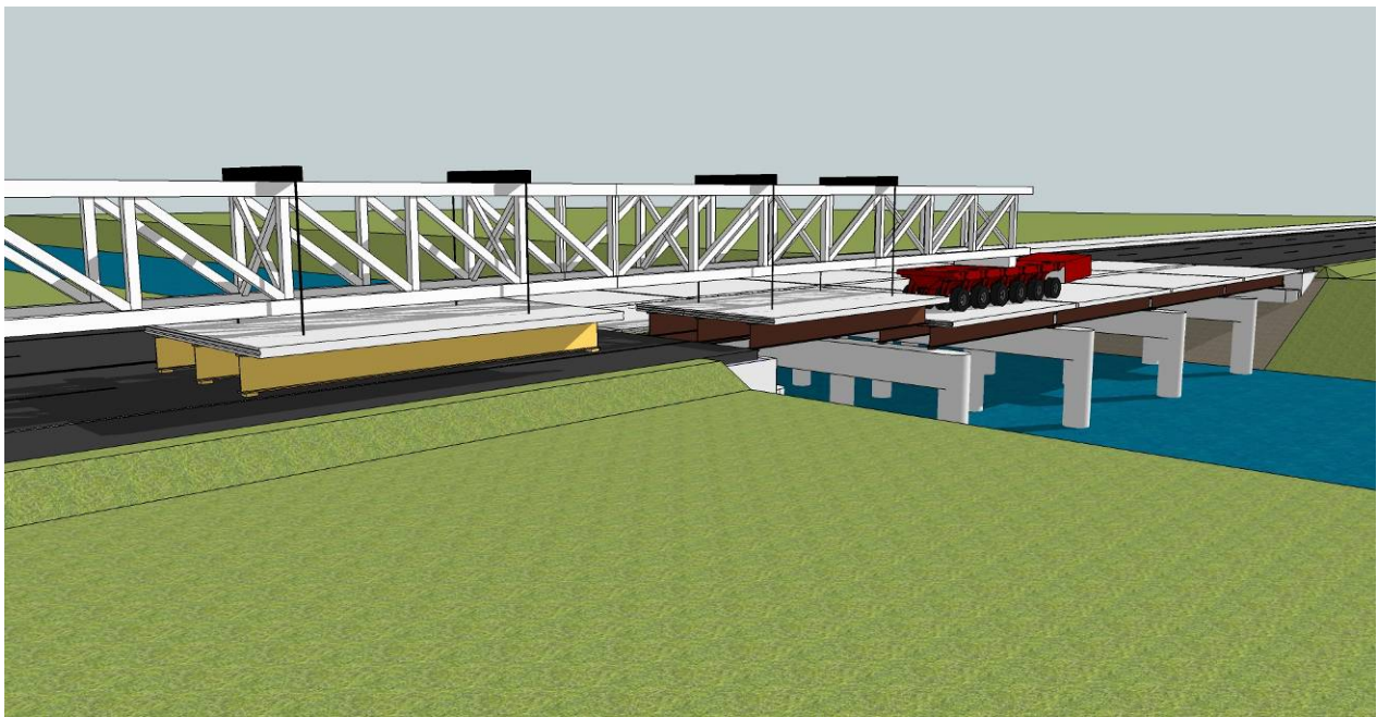
Installation of new Module using the Gantry Frame
