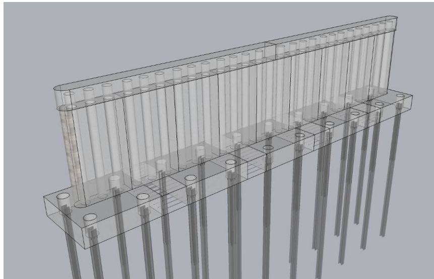
Figure A1.2-1 Precast Pier Supported on Piles
