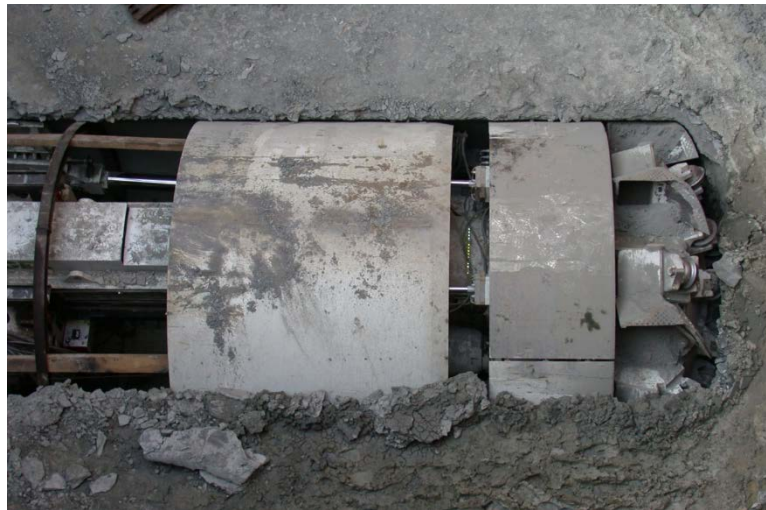
Figure 11. Photo. Cross section of pipe drilling machine, similar to a tunnel boring machine.
