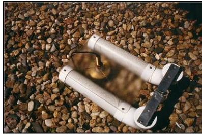
Figure 6-17 Transducer on Float
