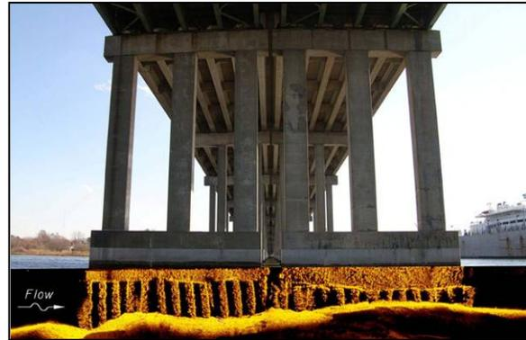
Figure 4-20 Acoustic Image of Concrete Pier with Steel Sheet Piling Cofferdam
