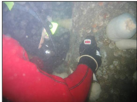
Figure 5-5 Waterproof Ultrasonic Thickness Measuring Device
