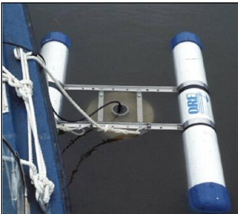
Figure 6-27 Low Frequency Transducer
