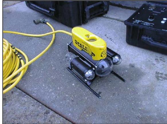
Figure 4-18 Remotely Operated Vehicle (ROV) with Control Console
