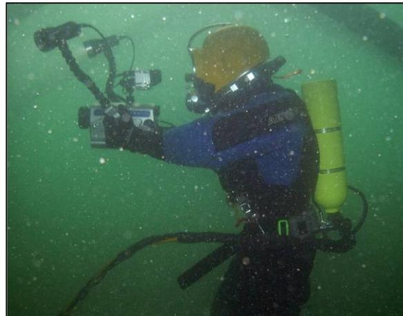
Figure 4-15 Video Camera in Housing with Monitor
