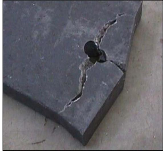
Figure 3-39 Failure of Composite Member
