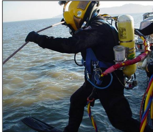
Figure 4-6 Diver Using Surface-Supplied Air with a Lightweight Helmet
