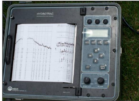
Figure 6-14 Hydrographic Survey Fathometer
