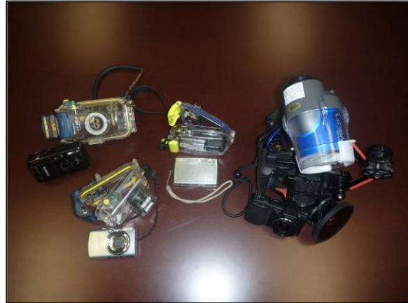
Figure 4-11 Various Waterproof Camera Housings
