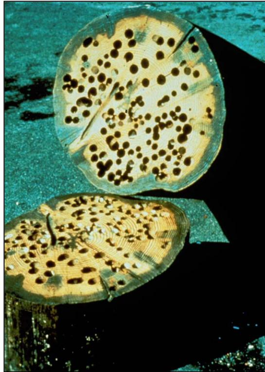
Figure 3-36 Timber Pile with Teredo Damage
