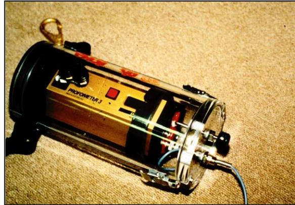
Figure 5-12 Rebar Locator in Waterproof Case
