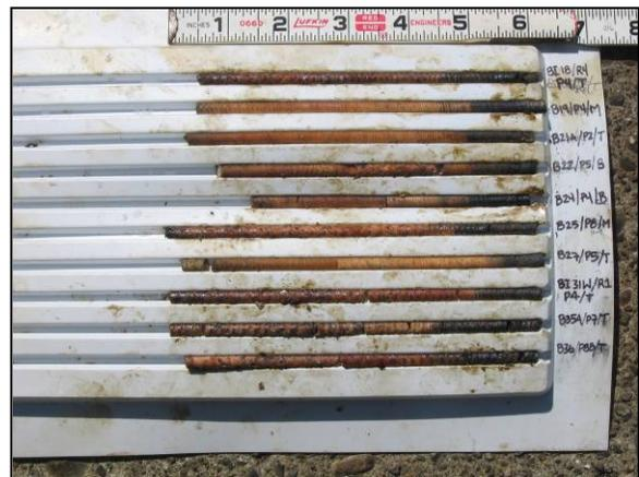
Figure 5-15 Timber Cores
