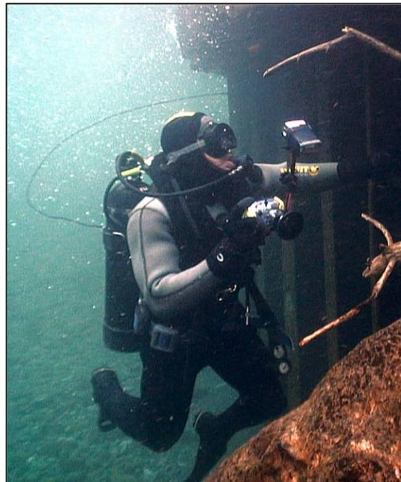
Figure 4-12 Digital Camera in Waterproof Housing
