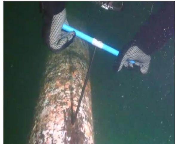
Figure 5-14 Diving Inspector Removing Timber Cores
