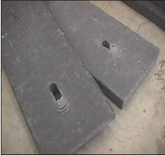
Figure 3-38 Yielding Around Hole of Composite Member
