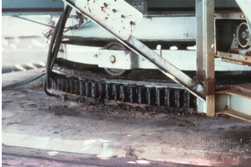
Figure 5.3.30 Balance Wheel in Place Over Circular Rack
