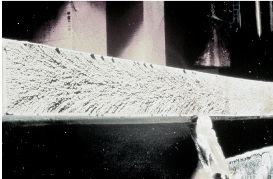
Figure 7.3.34 Brittle Fracture - Herringbone Pattern
