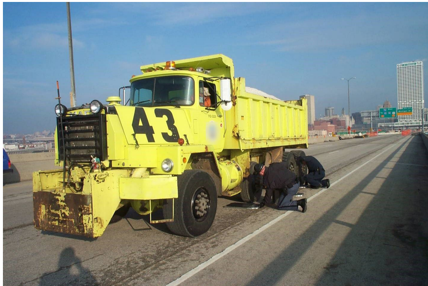
Figure 17.6.8 Dynamic Load Testing Vehicle
