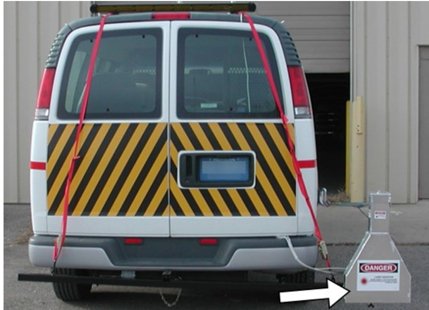
Figure 17.6.5 High Speed Underclearance Measurement System
