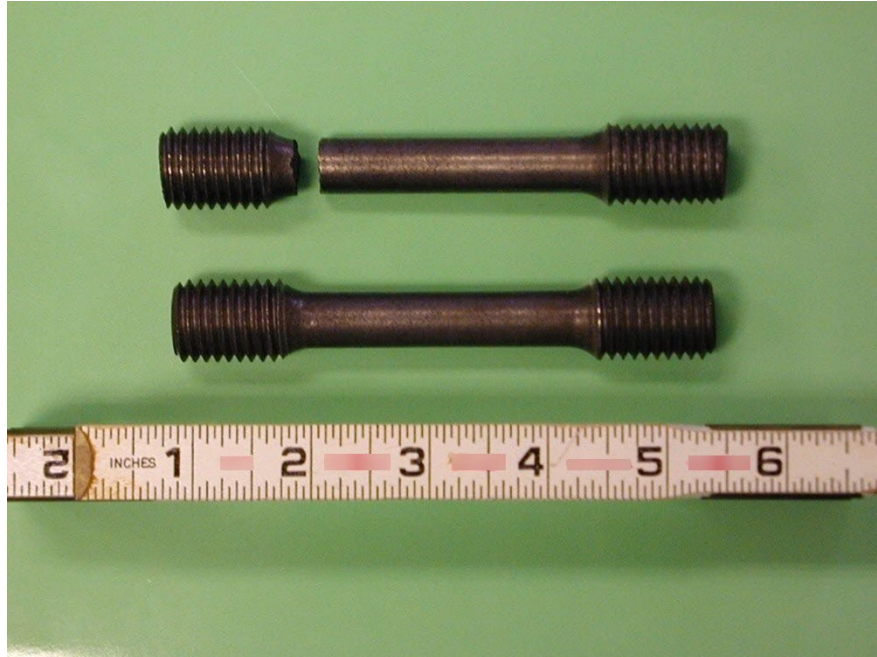
Figure 7.3.9 Brittle Fracture of Cast Iron Specimen
