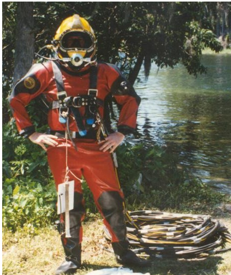
Figure 16.1.28 Surface Supplied Air Diving Equipment
