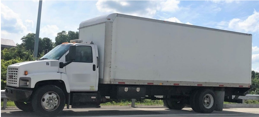
Figure 6.2.3 AASHTO H20 Design Truck and Similar Actual Truck
