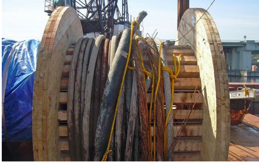
Figure 12.4.2 Frayed Cables Removed from a Floating Bridge
