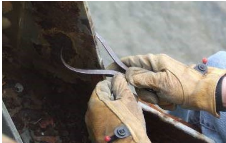
Figure 10.4.38 Using Calipers to Measure Gusset Plate Thickness
