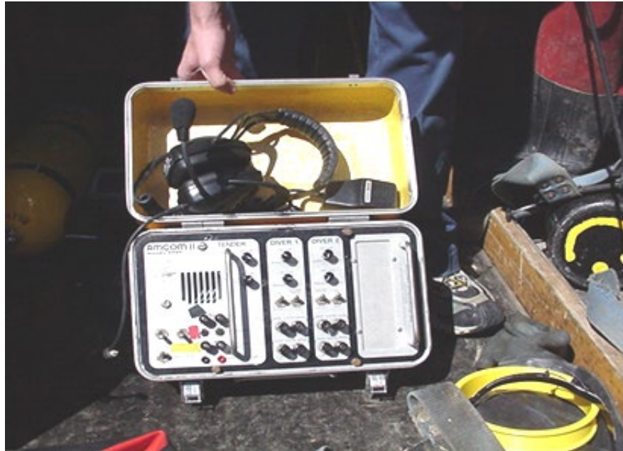
Figure 16.2.28 Wireless Communication Box System
