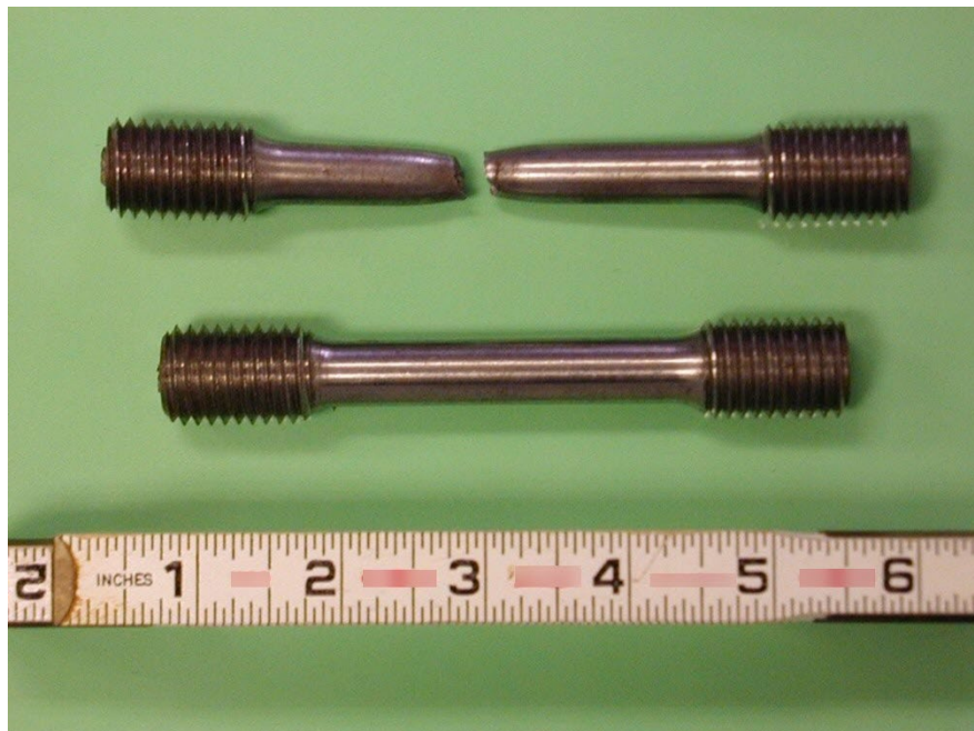
Figure 7.3.10 Ductile Fracture of Cold Rolled Steel Specimen
