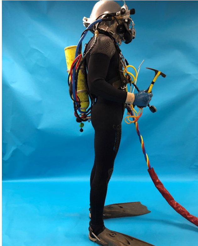
Figure 16.2.27 Surface-Supplied Diver with a Reserve Air Tank
