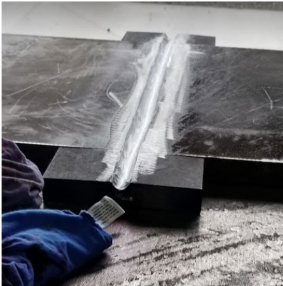
Figure 160. Photos. A backgouged and ground joint.
