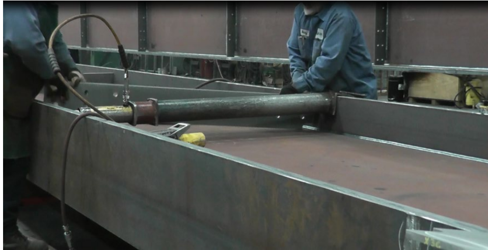
Figure 172. Photo. Girder flanges are commonly jacked to fit stiffeners.
