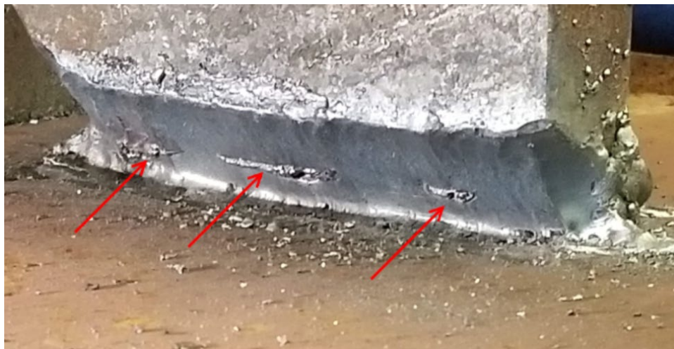
Figure 70. Photo. Example of slag trapped in a CJP weld
