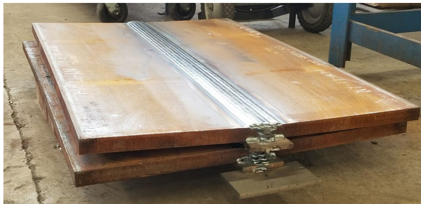
Figure 78. Photo. Angular distortion on groove qualification test plates.
