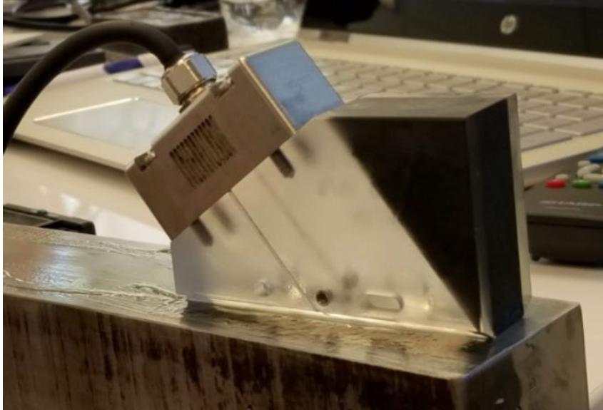
Figure 208. Photo and Illustration. Photo of transducer (left) and illustration of elements (right).
