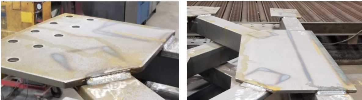
Figure 177. Photos. Gussets with clipped corners are preferred.
