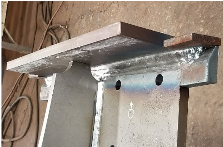
Figure 138. Photo. Weld tabs on a CJP weld T-joint.
