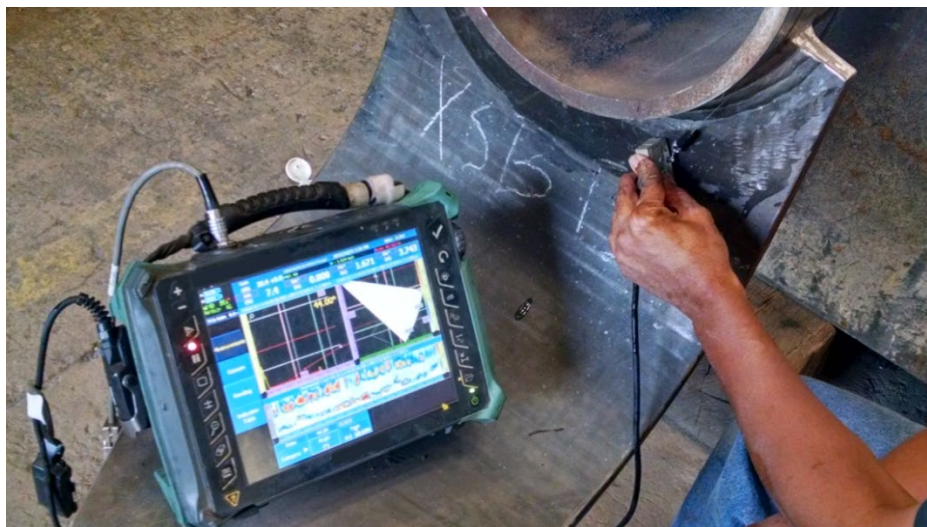
Figure 109. Photo. Use of PAUT for an unusual CJP bridge weld.
