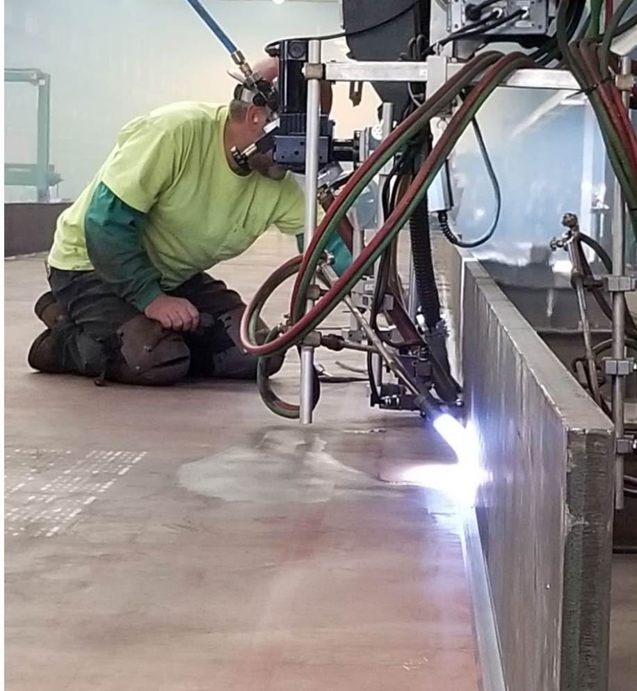
Figure 52. Photo. Preheat applied continuously ahead of welding.
