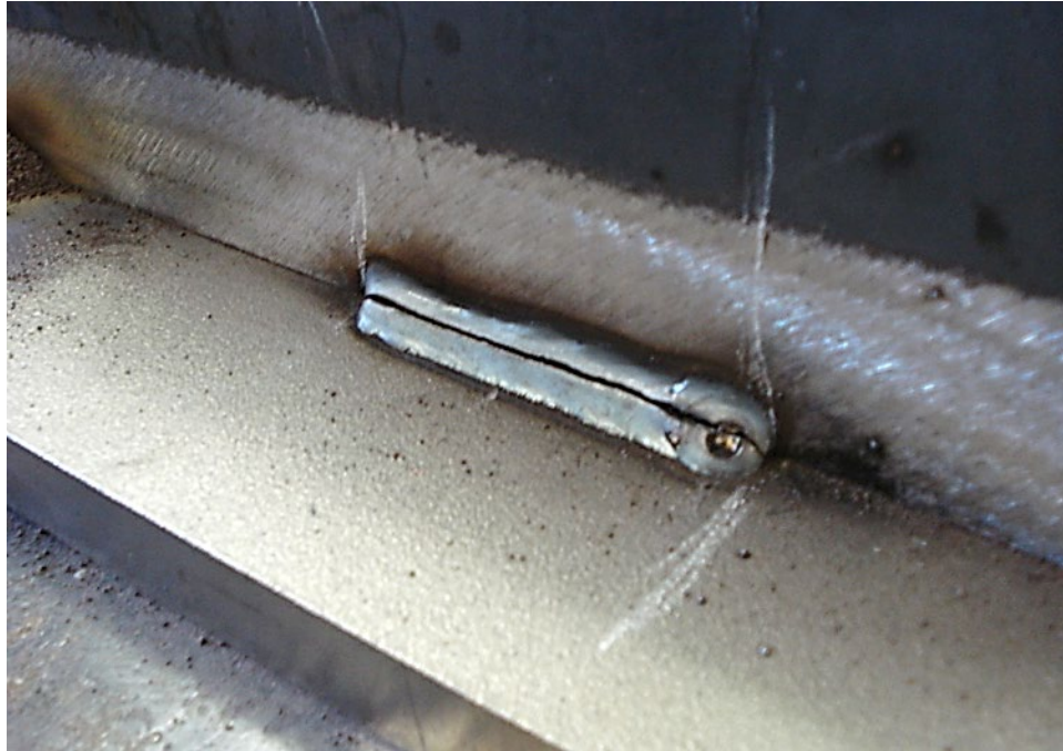
Figure 129. Photo. A broken tack weld, distinct from a cracked tack weld.
