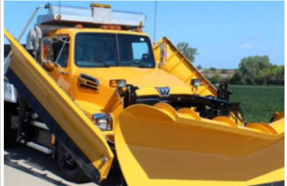
hydraulic system and spreader, 360-degree LED emergency lighting, LED wing lights, and rubber cutting plow edges with a blade saver on the front plow.
