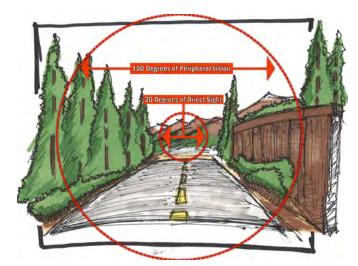
Figure 3-3: Drivers cone of vision at 55 mph
