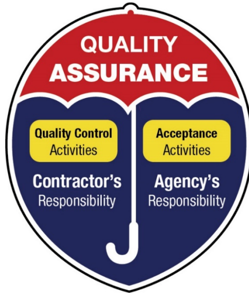
Figure 28. QA responsibilities: shared by the contractor and the agency.
