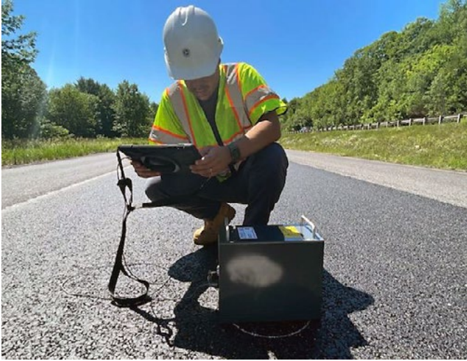
The MATC crew assesses the laboratory gyratory and field core macrotextures with field data collected using a laser texture scanner and a sand patch test. Source: FHWA
