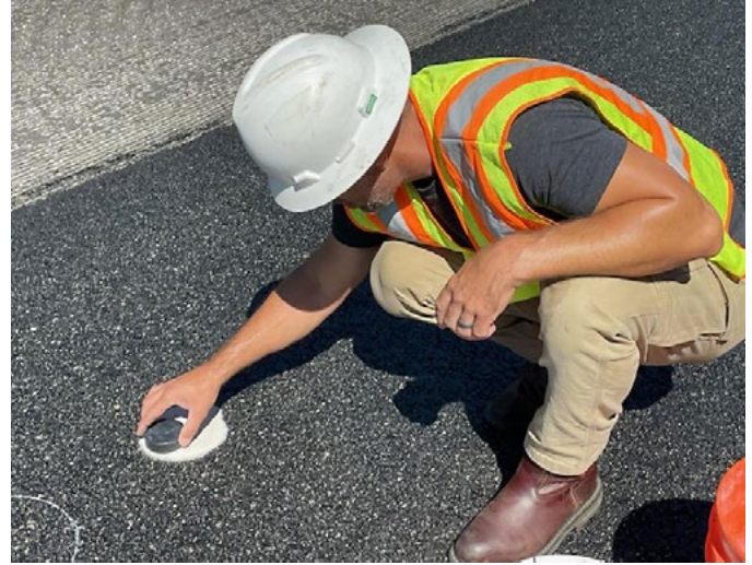
The MATC crew assesses the laboratory gyratory and field core macrotextures with field data collected using a laser texture scanner and a sand patch test. Source: FHWA
