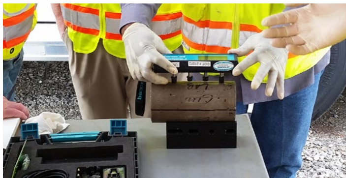
FHWA Mobile Concrete Technology Center technicians demonstrating the resistivity and SAM tests. Source: Shreenath Rao, ARA, Inc.
