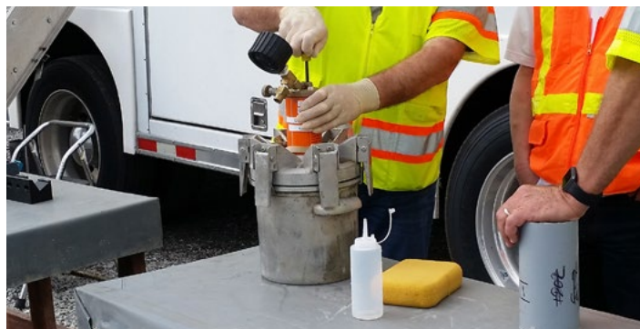
FHWA Mobile Concrete Technology Center technicians demonstrating the resistivity and SAM tests. Source: Shreenath Rao, ARA, Inc.
