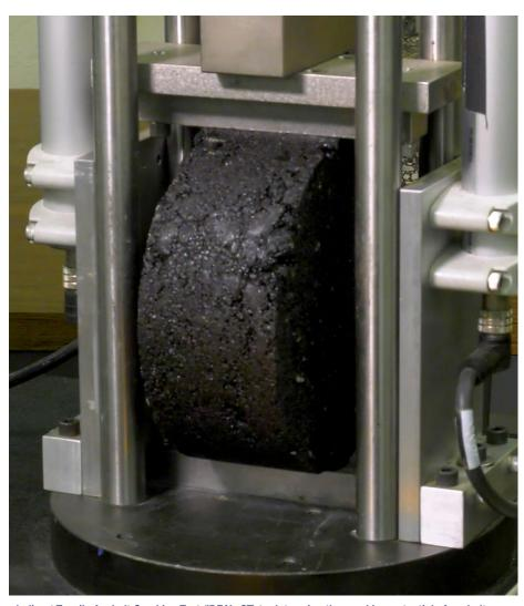
Indirect Tensile Asphalt Cracking Test (IDEAL-CT) to determine the cracking potential of asphalt mixtures. (Source: FHWA)
