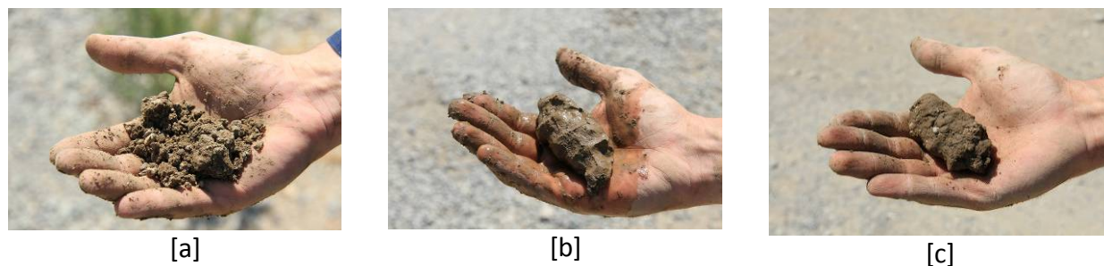
Figure 64. Photo. Squeeze test for assessing moisture content. ([a] too dry, [b] too wet, and [c] acceptable)
