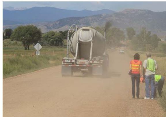
Figure 24. Photo. Acceptable dust level.
