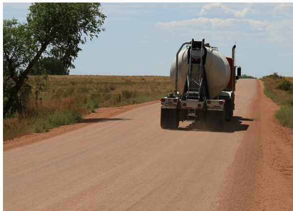
Figure 82. Photo. No dust. (1 on a scale of 1-5).
