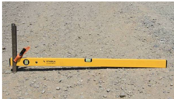
Figure 89. Photo. Checking crown with a simple level.
