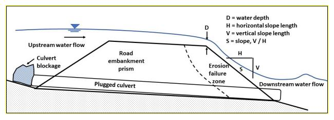
Figure 1. Road embankment with plugged culvert, failing due to overtopping (Provided by USFS)
