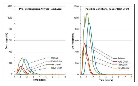
Figure 2. Pre-fire and post-fire discharge hydrographs (Provided by USFS)
