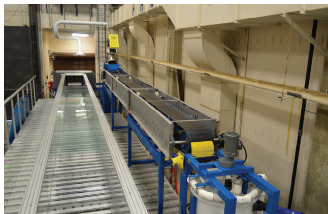
Photo 5—View of Conveyor Belt for Sediment Recirculation.
