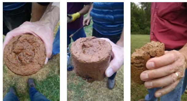
Figure 4—Eroded Soil Sample (Lean Clay) at 6.5ft
