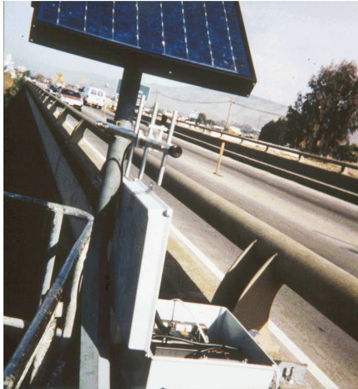
Figure 9.31. Typical instrument shelter with data logger, cell-phone telemetry, and a solar panel/gel-cell for power.
