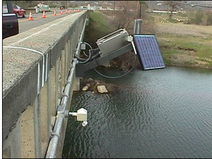
Figure 9.18. Tilt meter on California bridge.
