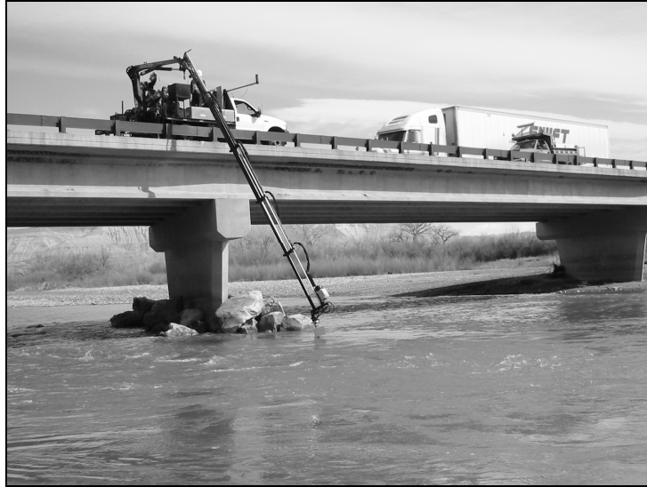
Figure 9.9. Sonar instrument deployed from articulated arm truck.
