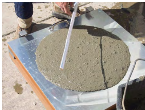
b. Measuring grout slump diameter
