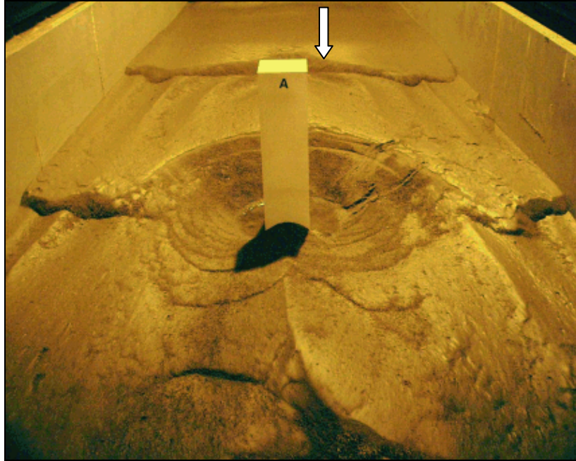
Figure 11.3. Unprotected square piers.
