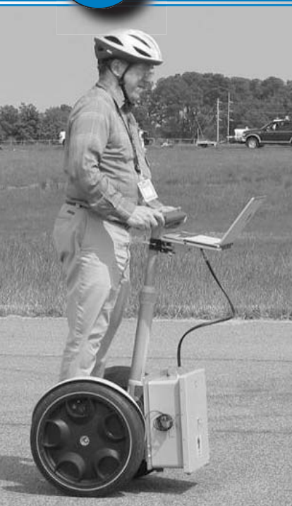
FHWA's profiler was built using a Segway Human Transporter.
