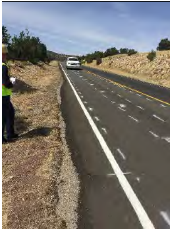
Figure 4. Photograph. Example of wheel path markings before the crack survey.
