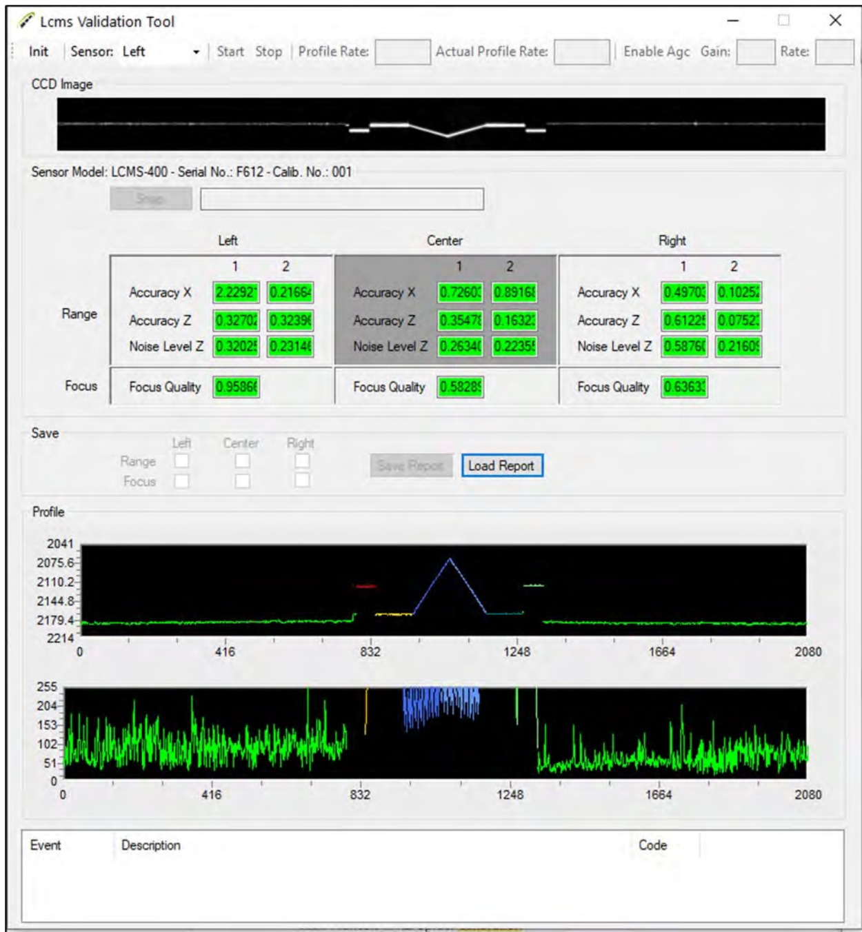
Figure 29. Illustration. Example of Validation Tool software being used to check data quality using the Validation Object.
