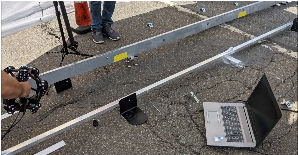
Figure 17. Photograph. Example of using hot glue to secure objects in place.
