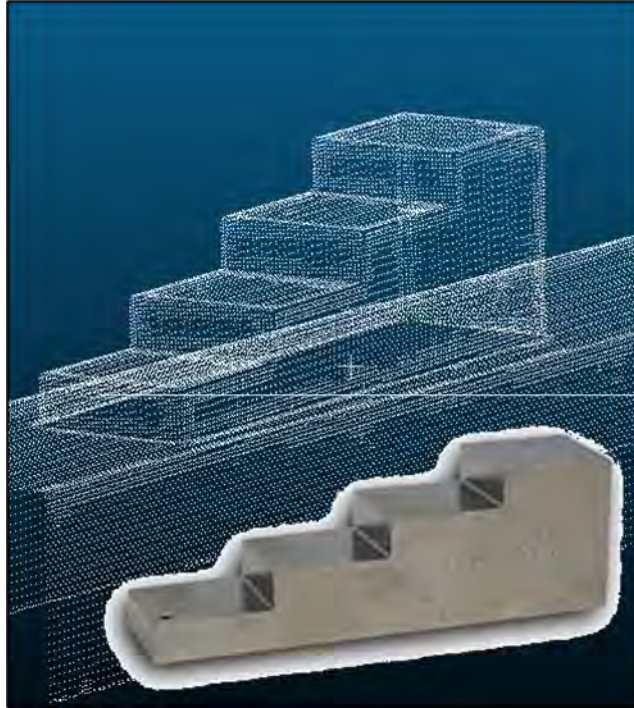
Figure 14. Illustration. Example data from a GRE scan of a stair-stepped gauge block.
