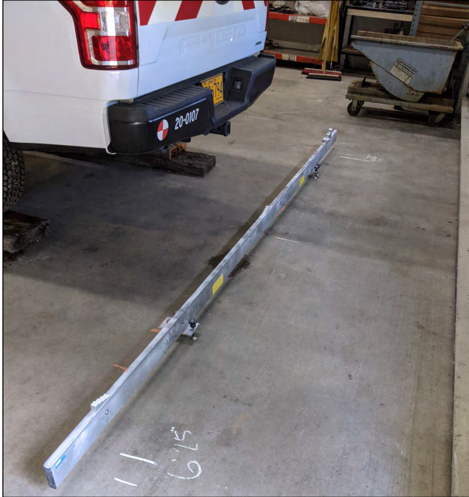
Figure 10. Photograph. Example of the straight edge with gauge blocks under mapping sensor.
