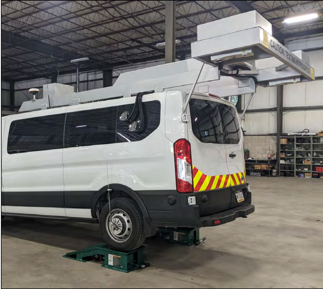
Figure 8. Photograph. Example of a raised test vehicle for the static test.
