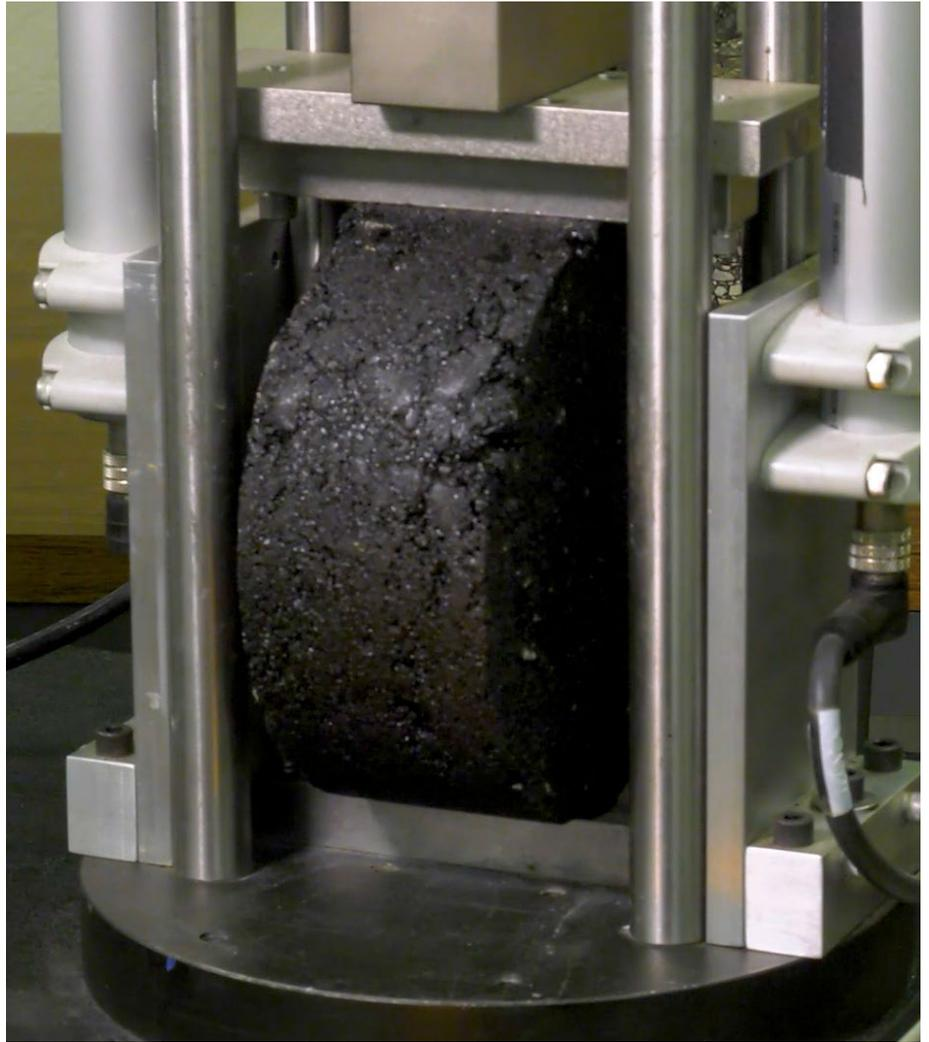
Indirect Tensile Asphalt Cracking Test (IDEAL-CT) to determine the cracking potential of asphalt mixtures. (Source: FHWA)
