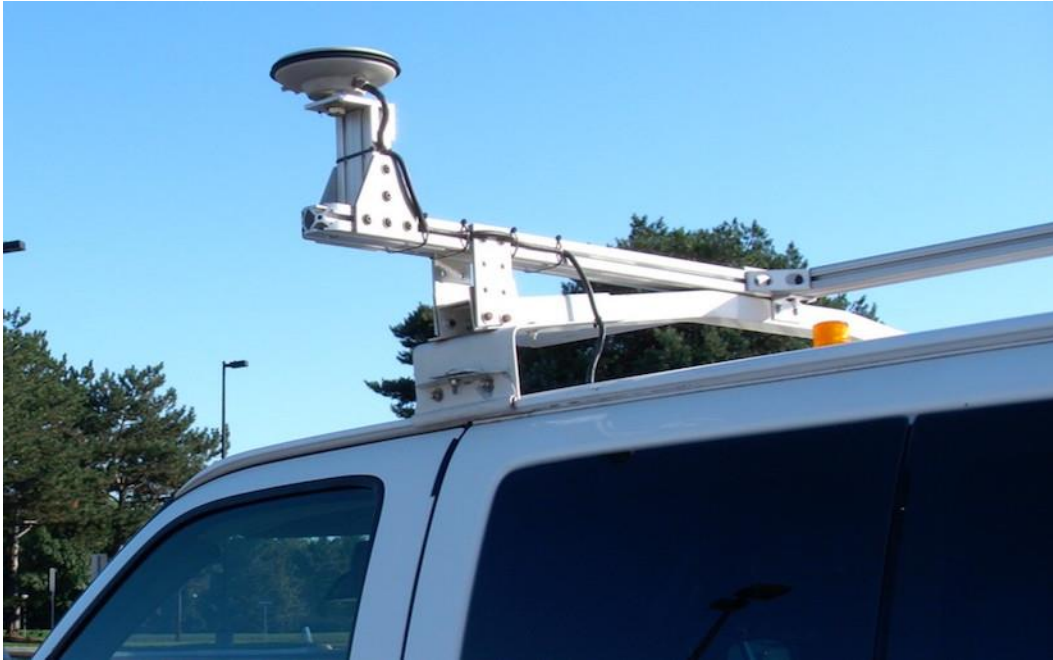
Figure 211. Image. Front left GPS antenna (pitch rover).
