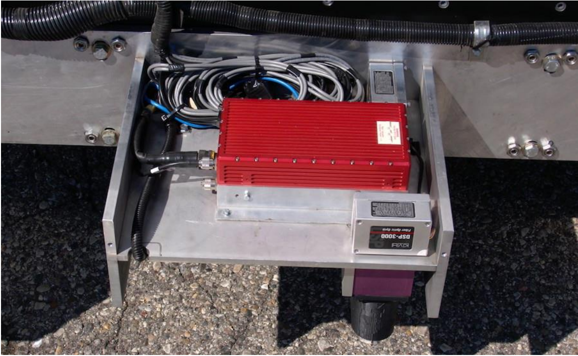
Figure 209. Image. Center sensor pod, cover removed.
