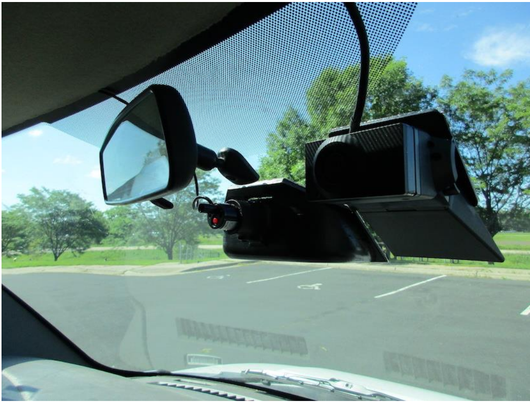
Figure 210. Image. Forward camera and lane tracker camera.
