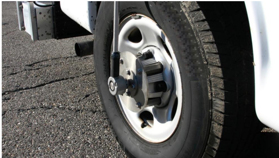
Figure 206. Image. Rotational encoder mounting hardware.
