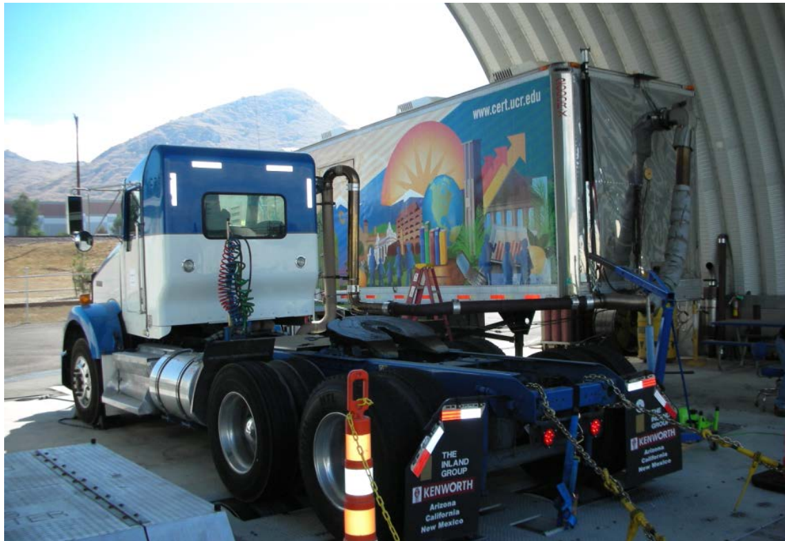
Figure 5-7. Truck being tested on the chassis dynamometer
