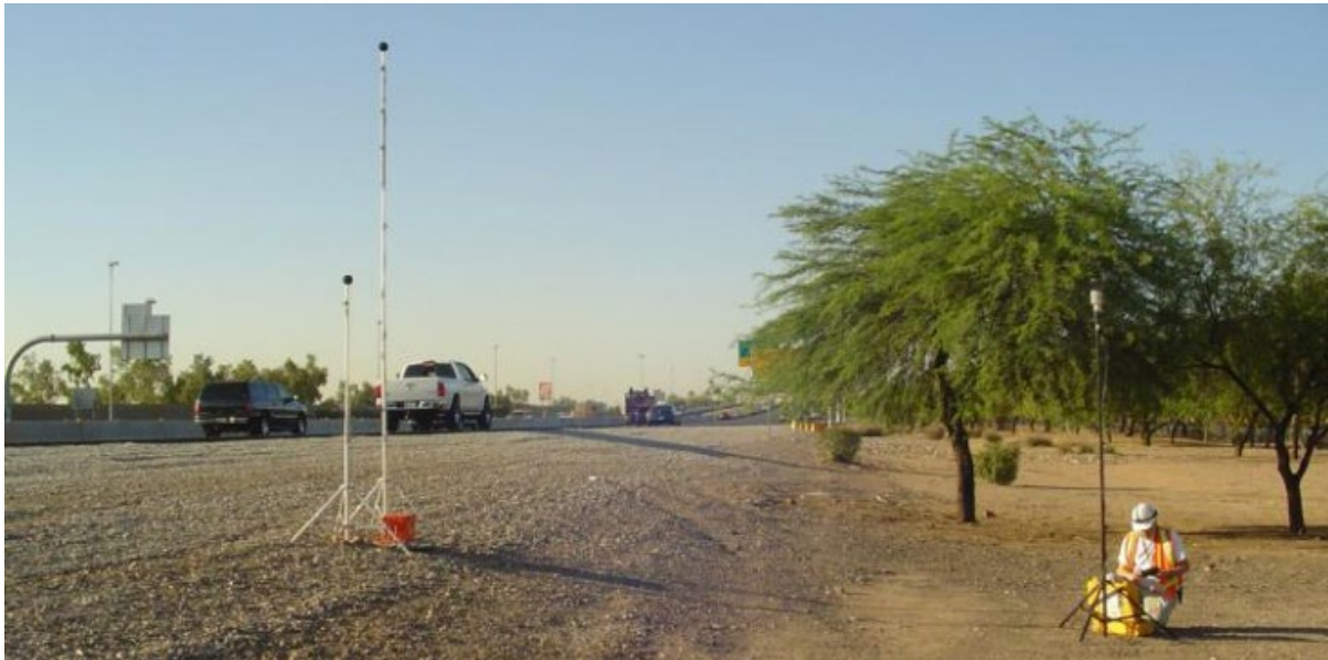
FIGURE 4 CTIM METHOD EQUIPMENT SETUP (Photographic References: PR_04)
