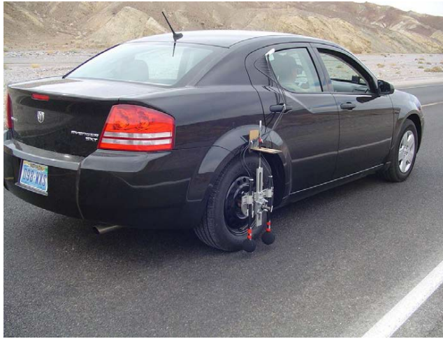
FIGURE 8 OBSI METHOD EQUIPMENT SETUP (Photographic References: PR_02)
