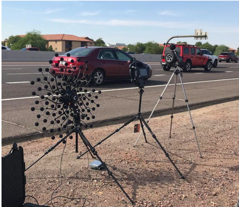
FIGURE 6 ACOUSTIC CAMERA METHOD EQUIPMENT SETUP (Courtesy of Ivan Racic of the Arizona Department of Transportation)
