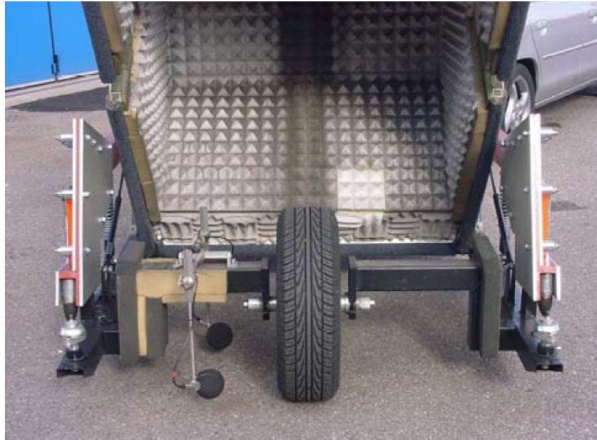
FIGURE 7 CPX METHOD EQUIPMENT SETUP (Photographic References: PR_03)
