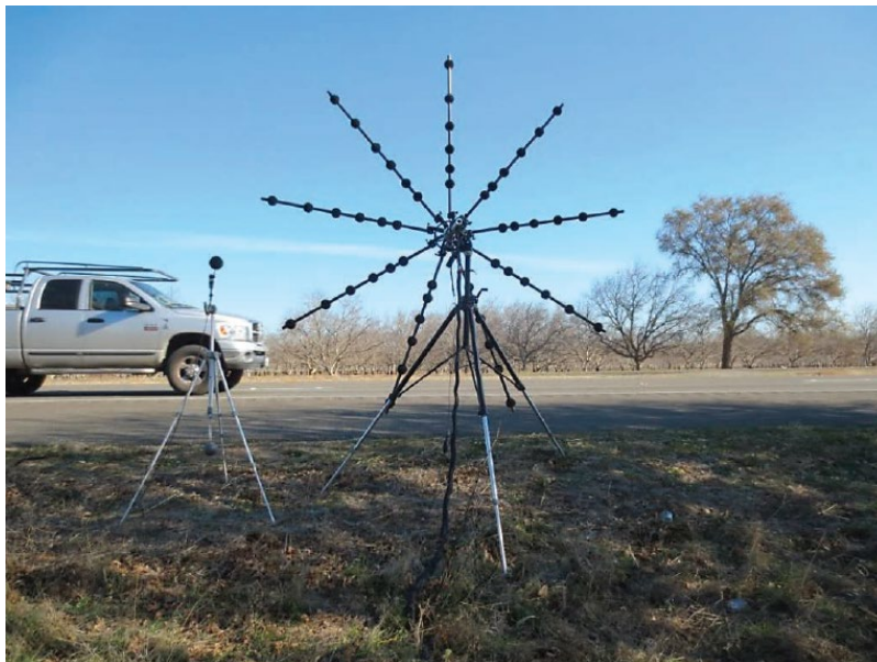
FIGURE 9 BEAMFORMING ARRAY AND SINGLE SOUND LEVEL METER MEASURING VEHICLE PASS-BY (Photographic References: PR_06)
