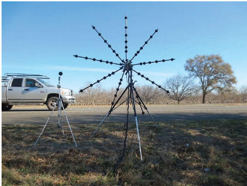
FIGURE 5 EXAMPLE BEAMFORMING EQUIPMENT SETUP 9 (Photographic References: PR_06)
