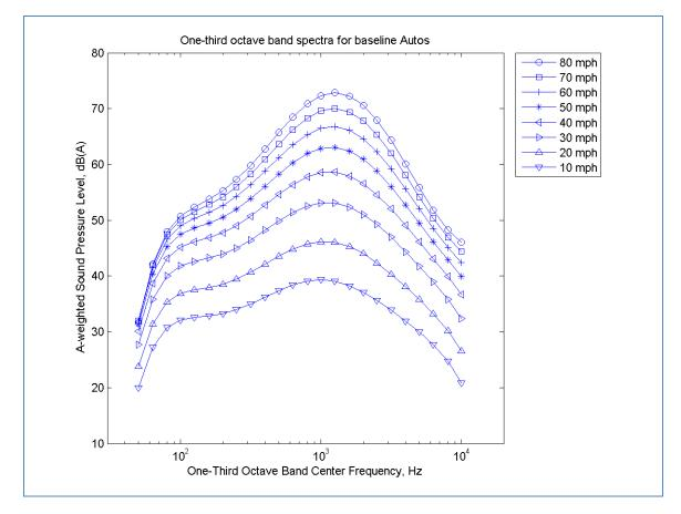
Figure 2: A-weighted Spectral Shape According to REMEL Model
