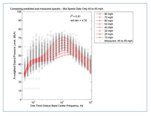
Figure 17: Example of Spectral Modeling Using only Mid Speed Data – 45 to 65 mph
