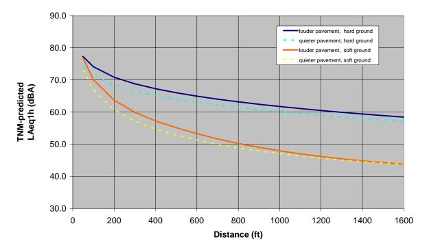
Figure 1. TNM-predicted sound pressure levels (L<sub>Aeq1h</sub>) as a function of distance – flat site, no noise barrier. Variables: louder and quieter pavement, acoustically hard and soft ground.
