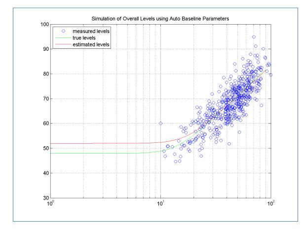
Figure 11: True and Estimated Models – No Low Speed Data
