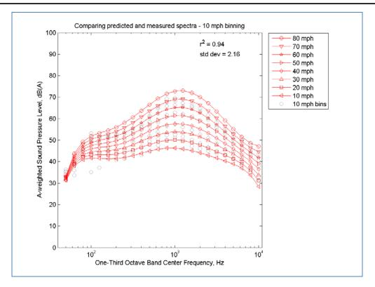
Figure 22: Spectral REMELs Derived from 10 mph Speed Bins
