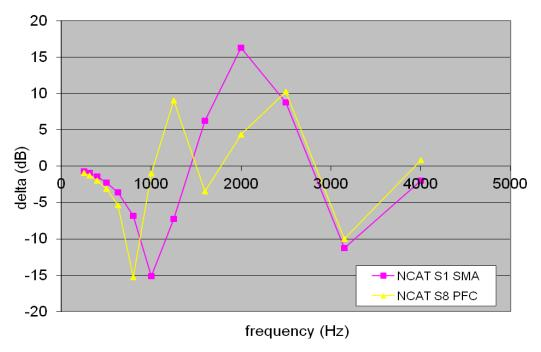
Figure 14. Example measured EFR curves, typical and atypical.
