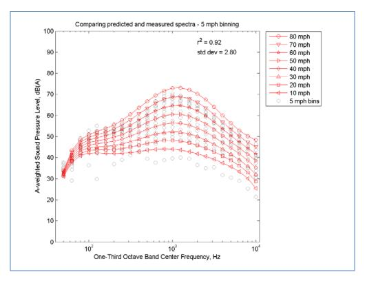
Figure 21: Spectral REMELs Derived from 5 mph Speed Bins
