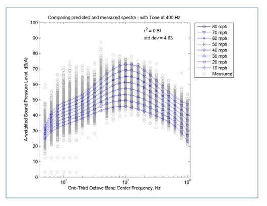
Figure 23: Example of REMEL Spectra and Underlying Data with Tonal Component
