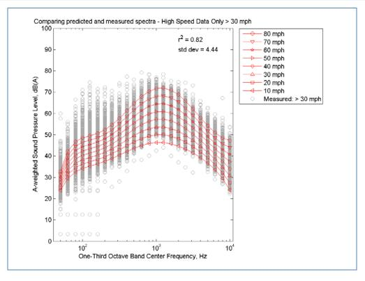
Figure 19: Example of Spectral Modeling Using only High Speed Data > 30 mph
