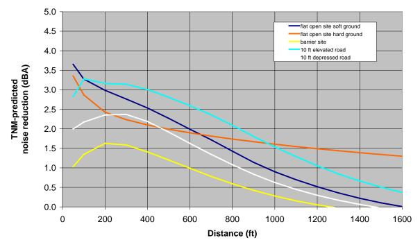
Figure 2. TNM-predicted noise reductions (L<sub>Aeq1h</sub> for louder pavement minus quieter pavement) as a function of distance. Variables: flat site (with acoustically hard and soft ground), barrier site, elevated road, depressed road.
