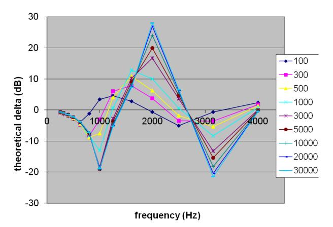
Figure 12. Example theoretical EFR curves. For each EFR value (cgs rayls), the data are presented as the delta sound level between the two microphones (upper minus lower) as a function of frequency.
