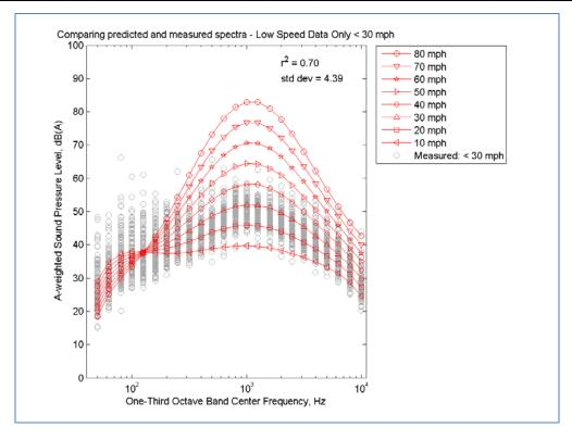
Figure 15: Example of Spectral Modeling Using only Low Speed Data < 30 mph
