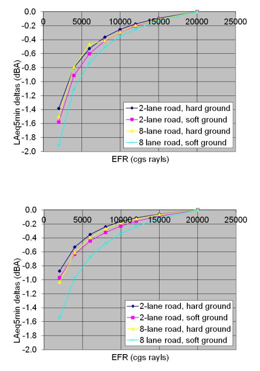
Figure 9. Sound level differences from that for 20K EFR as a function of EFR; 2- and 8lane road, hard and soft ground. Top plot: distance = 50 ft, bottom plot: distance = 200 ft.
