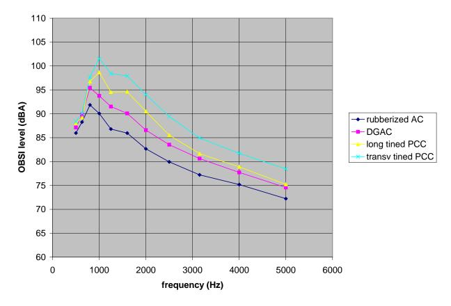
Figure 5. Plot of average OBSI data for each pavement type used for proof-of-concept study.
