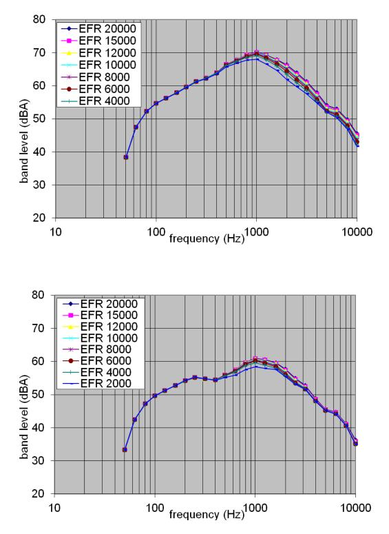
Figure 10. Spectral sound levels with varying EFR values; 8-lane road, soft ground. Top plot: distance = 50 ft, bottom plot: distance = 200 ft.
