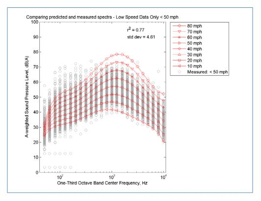
Figure 16: Example of Spectral Modeling Using only Low Speed Data < 50 mph
