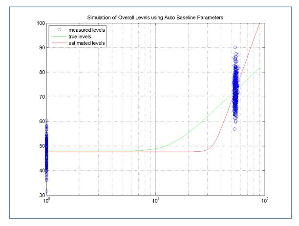
Figure 13: True and Estimated Models – Not Enough Range on High Speed Data
