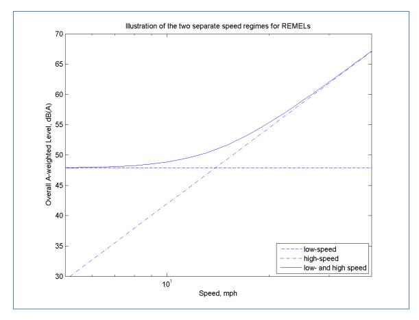
Figure 1: Overall A-weighted Level According to REMEL Model
