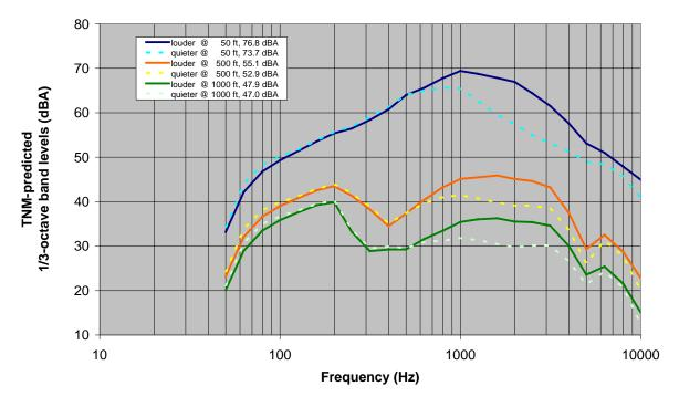
Figure 3. TNM-predicted sound pressure spectral levels (LAeq1h) – flat site, no noise barrier, acoustically soft ground. Variables: distance, louder and quieter pavement.
