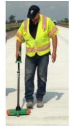
Metal 'Target' (2.5" to 12.5" dia) MIT Scan T2
