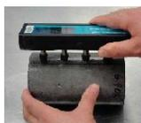
**Summary:** Permeability of concrete impacts its long-term durability. The SR method offers agencies reduced testing time, effort, and cost for assessing concrete permeability compared to the RCPT. This technology can also be used for Quality Control by contractors for assessing the quality of their concrete. Quantified benefits of this technology (agency and industry) for one state (Louisiana) are published in Reference 1.
