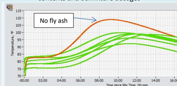
Significant difference in Heat Signature curve (yellow) due to no-fly ash in the sample
