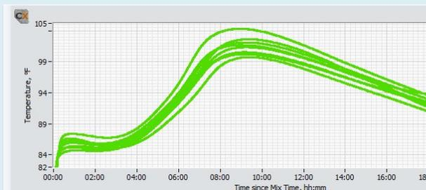
Consistent Heat Signature Curves from a field project with consistent quantities and sources of cementitious contents and admixture dosages
