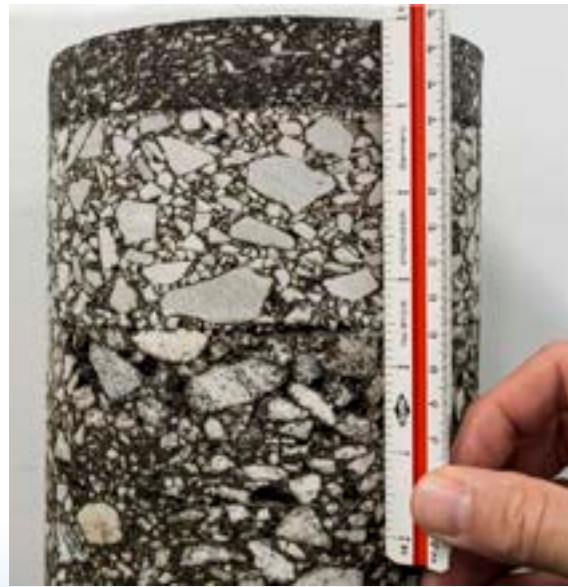
(Above) This asphalt pavement core shows a fine-graded, 1-inch overlay on top of the original pavement structure.
