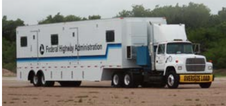
The Mobile Asphalt Testing Trailer is one tool FHWA uses to encourage interaction with State DOTs, introducing innovations, new technology, and test methods to pavement engineers across the United States. Source: FHWA.
