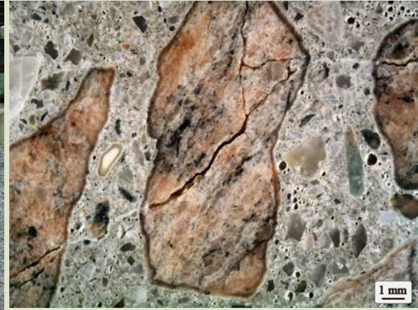
Concrete foundation of a storage tank in Hurt, Virginia constructed in 1993 (left). Close-up view of ASR-distressed concrete (right). Coarse aggregate is a granitic gneiss. Photo sent by Nick Scaglione, Concrete Research and Testing, LLC.
