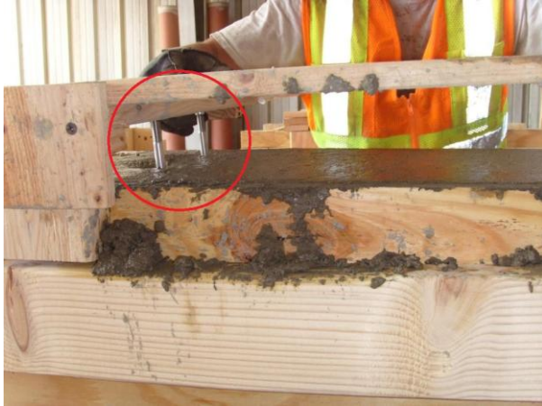
Figure 7. Placing wood formwork with steel pins into the top of the fresh concrete. The pins will be used to monitor the expansion of the block.
