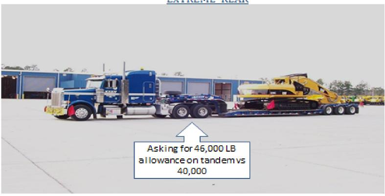
LOAD = CAT 329 EXCAVATOR LOAD WEIGHT = 67,262 L6 HEIGHT = 13.6' WIDTH = 11' 2" TOTAL LENGTH = 75' OOO O O O 10,500
