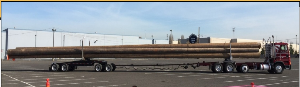
ODOT images: Tractor with 70' logging trailer and 102' long load, Total Length=112' and Tractor with 101' booster trailer, Total Length=125'
