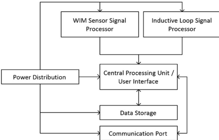
Figure 26 – WIM Controller Internal Components Functional Diagram
