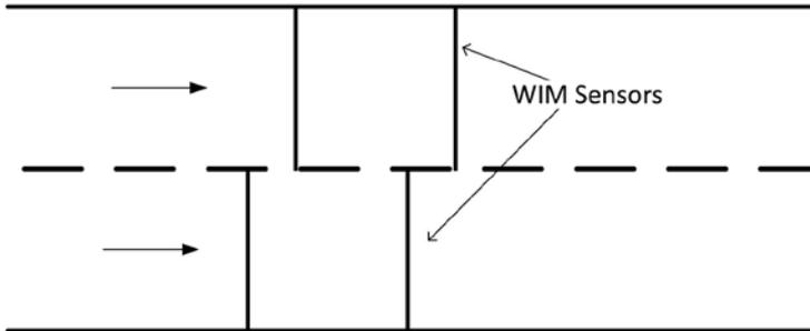
Figure 25 – 2-Lane Unidirectional Portable Piezo Full Lane Width Sensors
