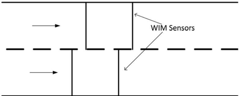
*Figure 9 – 2-Lane Unidirectional Bending Plate In-Line Sensor Configuration*
