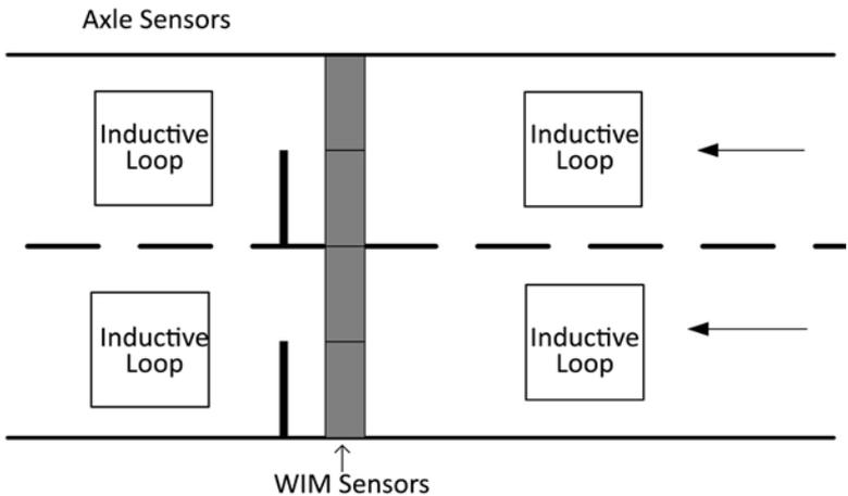
*Figure 13 – 2-Lane Unidirectional In-Line Load Cell Configuration*
