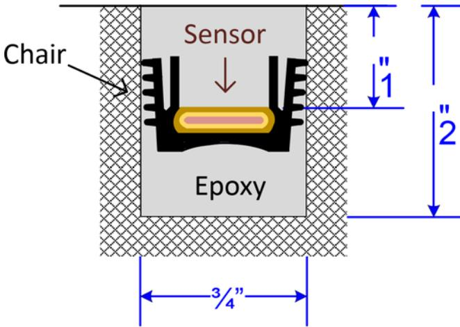
Figure 16 – Polymer Piezo Installation Depiction
