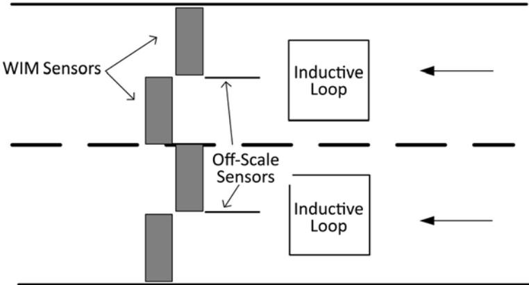
Figure 14 – 2-Lane Unidirectional Staggered Load Cell Configuration
