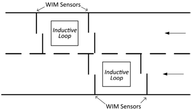
Figure 17 – 2-Lane Unidirectional Polymer Piezo 2-Sensors per Lane Configuration
