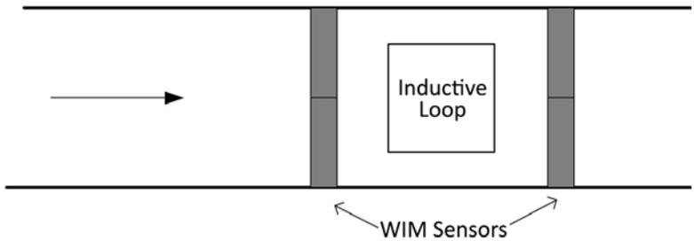
*Figure 10 – Single Lane Type III Sensor Configuration*
