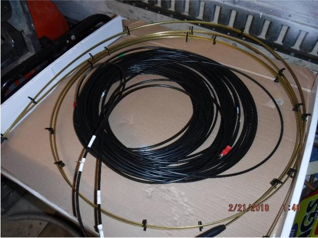
Figure 15 – Polymer Piezo Sensor
