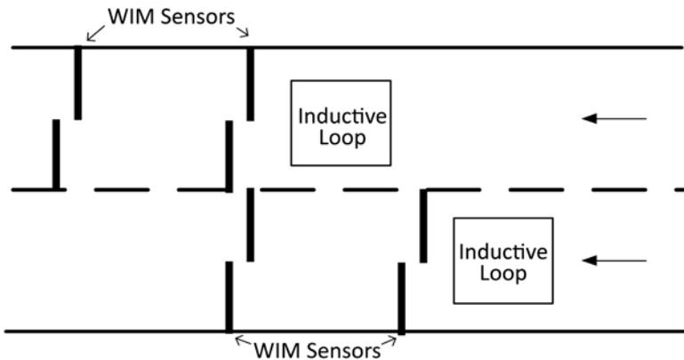
Figure 22 – 2-Lane Unidirectional Strain Gauge Strip Sensor Staggered Double Threshold Configuration
