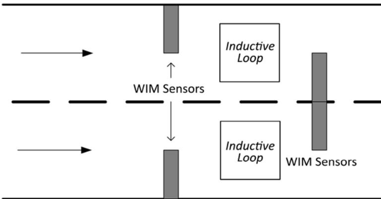
Figure 8 – 2-Lane Unidirectional Bending Plate – Staggered Configuration
