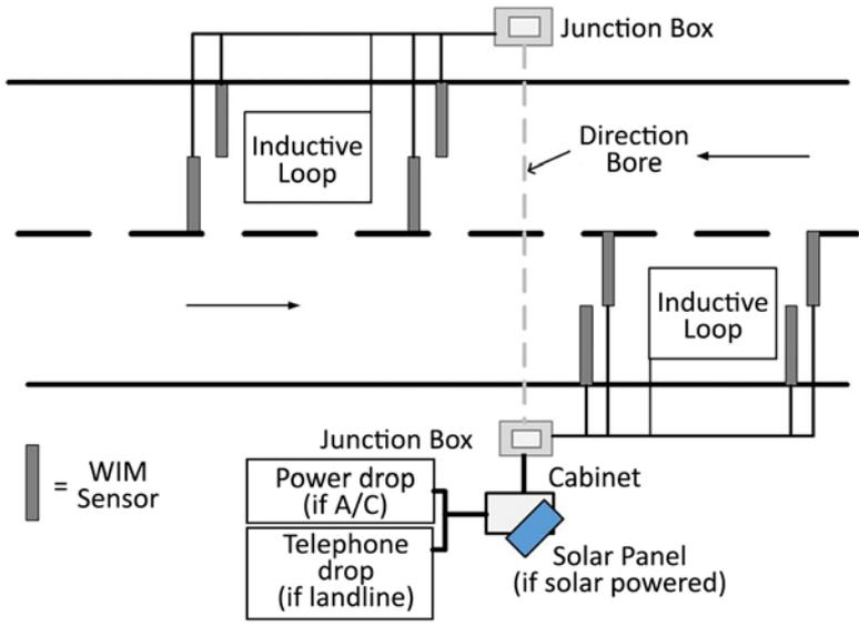
Figure 1 – Typical 2-Lane Bidirectional WIM System Design
