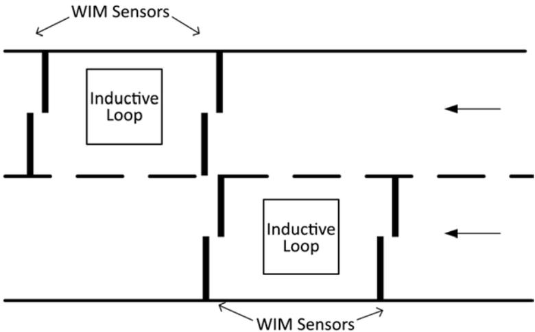
Figure 20 – 2-Lane Quartz Piezo Sensors Staggered Double Threshold Configuration
