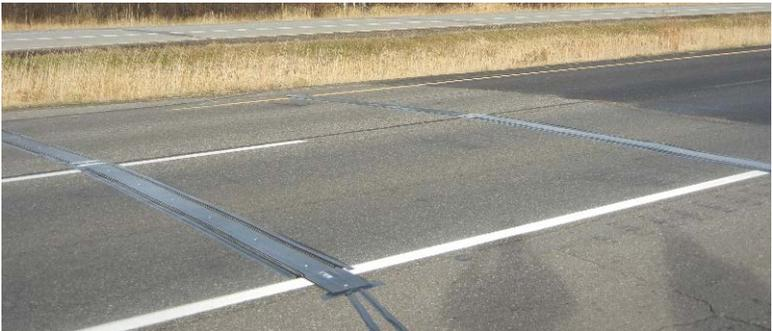
*Figure 24 – Single Lane Portable WIM Sensor*
