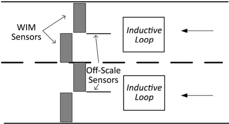
*Figure 10 – 2-Lane Unidirectional Staggered Load Cell Configuration*
