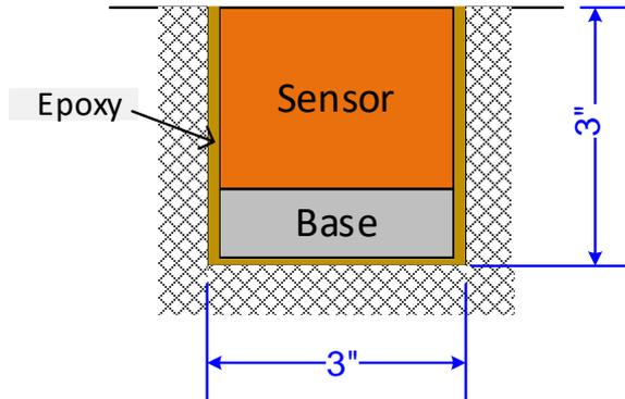
Figure 13 – Strain Gauge Strip Sensor Installation Detail
