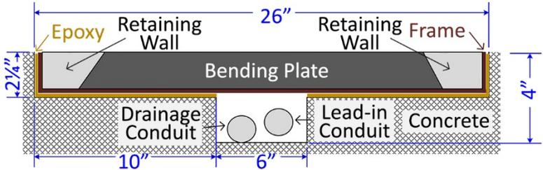
Figure 6 – Bending Plate Installation Detail
