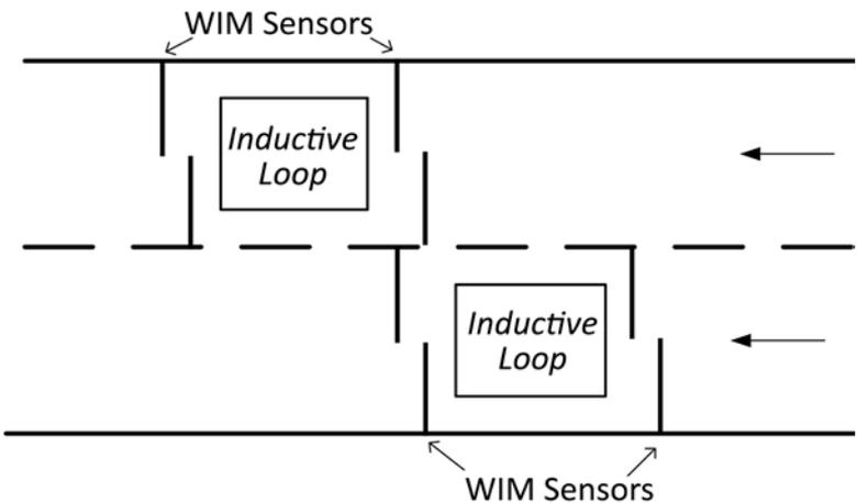
*Figure 16 – 2-Lane Unidirectional Polymer Piezo 4-Sensor per Lane Configuration*
