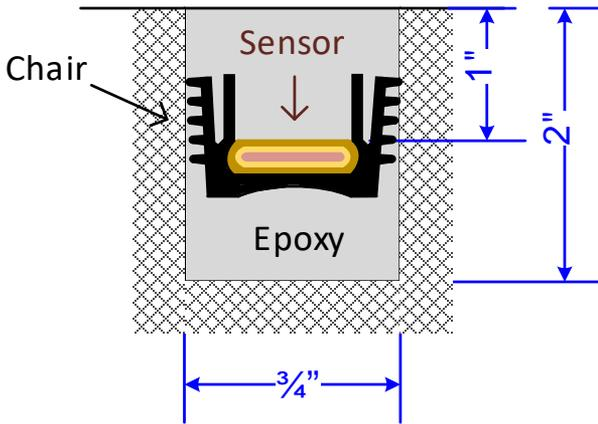
Figure 15 – Polymer Piezo Installation (not to scale)
