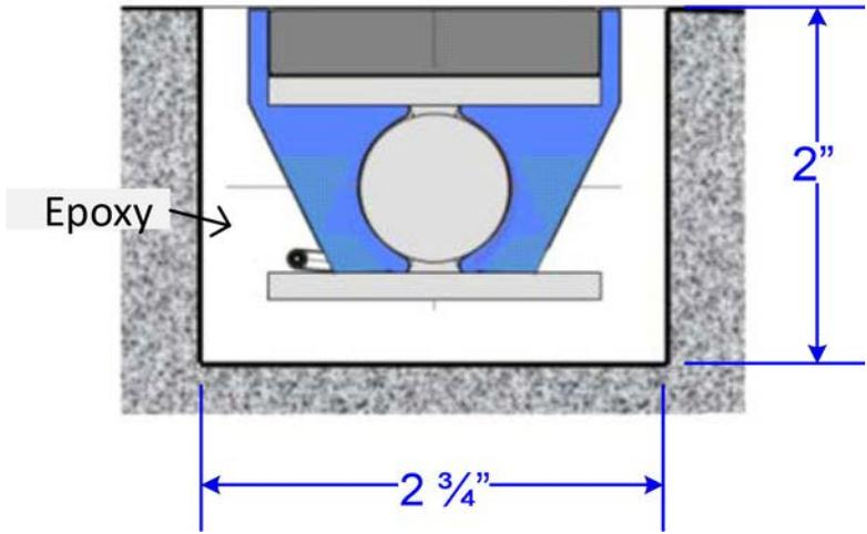
*Figure 11 – Quartz Piezo Installation Detail*
