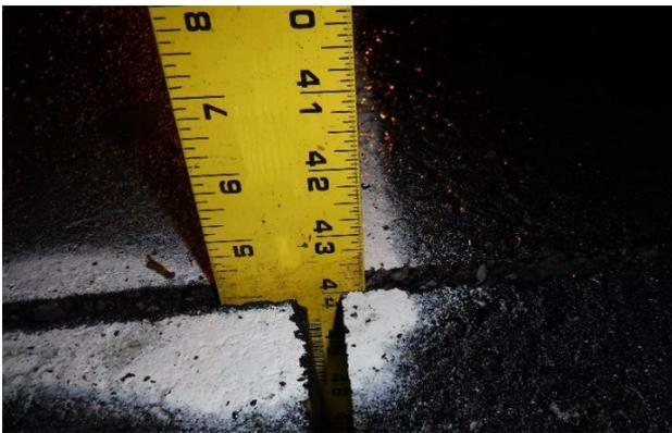
*Figure 39 – Slot Depth Measurement*
