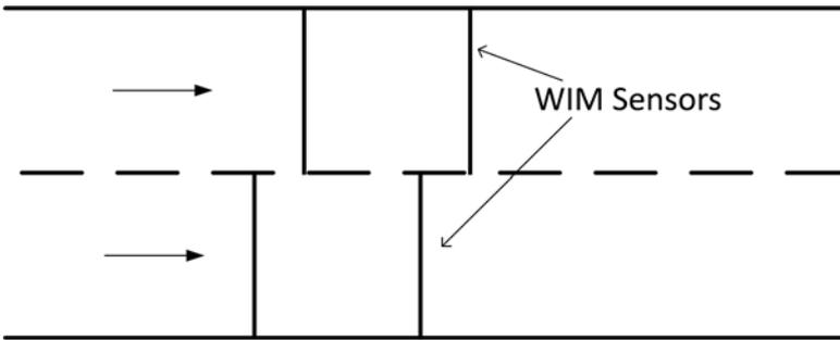
*Figure 17 – 2-Lane Unidirectional Portable Polymer Piezo 2-Sensor per Lane Configuration*
