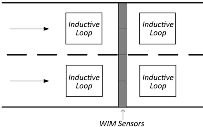
*Figure 8 – 2-Lane Unidirectional In-Line Bending Plate Configuration*
