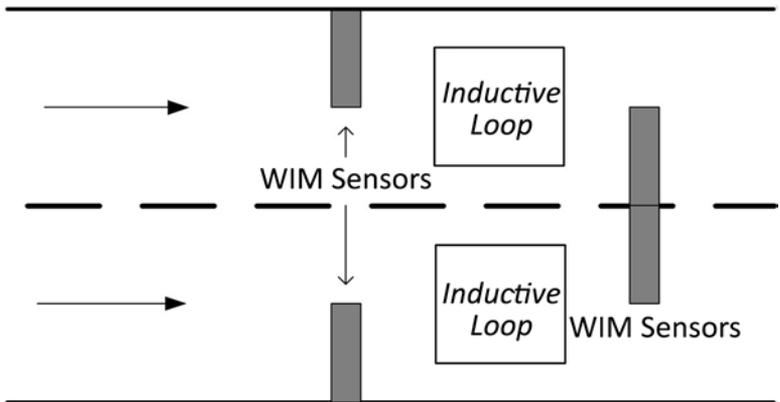
Figure 7 – 2-Lane Unidirectional Staggered Bending Plate Configuration
