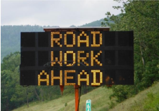
Figure 32 – Portable Changeable Message Sign Used for Traffic Control
