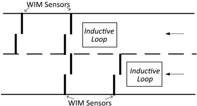
Figure 14 – 2-Lane Unidirectional Staggered Strain Gauge Strip Sensor Configuration
