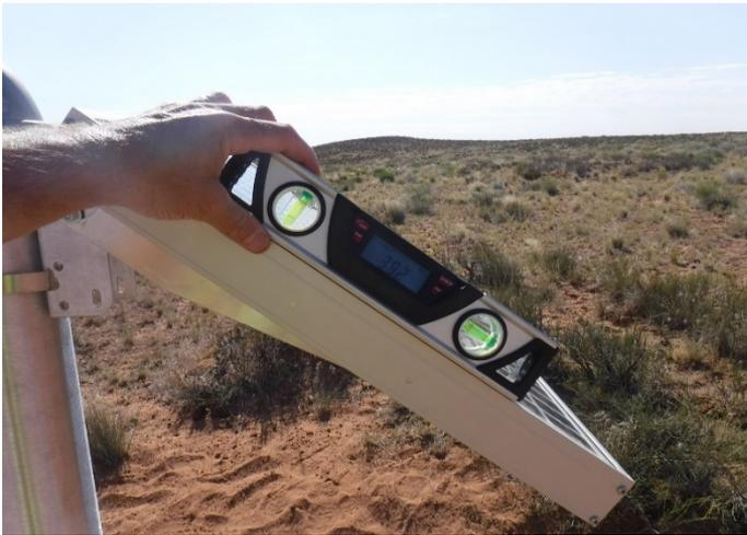
*Figure 35 – Solar Panel Angle Check*
