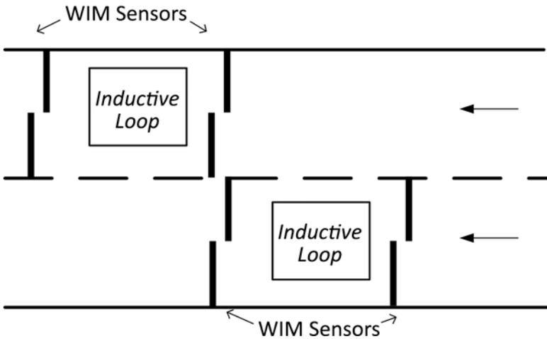
Figure 12 –2-Lane Unidirectional Staggered Quartz Piezo Configuration
