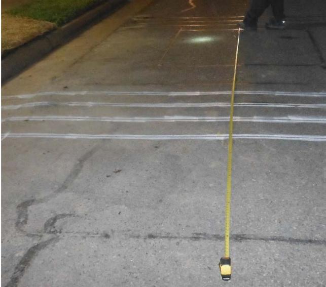
*Figure 37 – Loop Separation Measurement*
