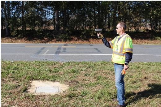
*Figure 12 – Collecting Test Truck Speed*
