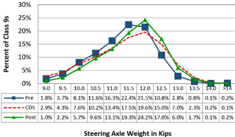
Figure 14 – Example of Post Visit Analysis of Class 9 Steering Axle Weight Distribution
