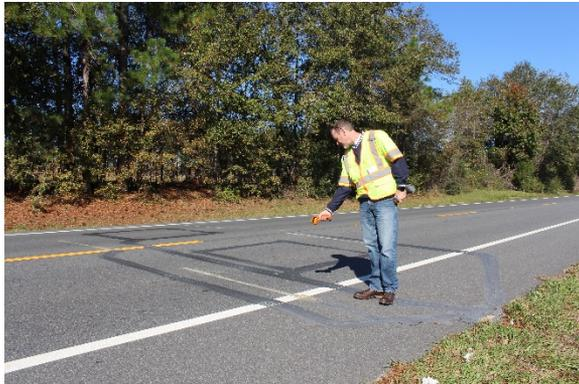
*Figure 13 – Collecting Pavement Temperature*
