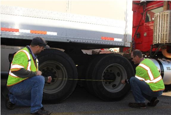
*Figure 2 – Measuring Test Truck Axle Spacing*
