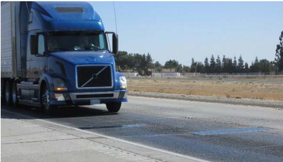
*Figure 1 – Calibration Test Truck Approaching WIM Scale*
