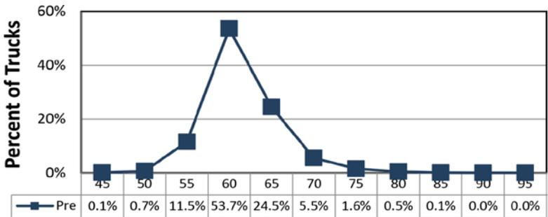
Figure 7 – Truck Speed Distribution Plot
