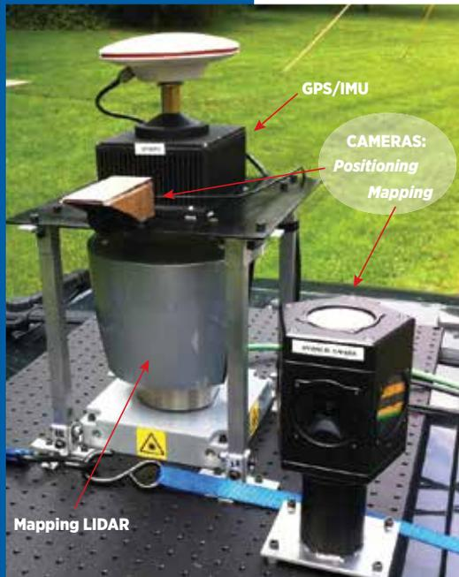
Feature-based mapping and positioning sensor suite showing a GPS/IMU (inertial measurement unit) box and a forward-looking camera for positioning, and a 360-degree camera and Velodyne® LIDAR for mapping.
