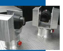
Cameras that can cooperate using precise and fast electronic pan, tilt, and zoom gimbals for event detection.
