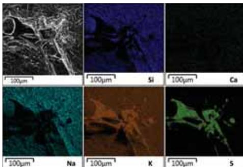
Backscattered electron images of a potassium sulfate crystal formed inside of a silica gel in the interfacial transition zone.
