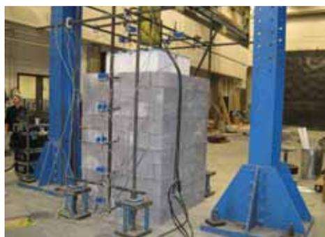
Minipier tests helped quantify SLS for GRS with (upper photo) and without (lower photo) concrete masonry facing.
