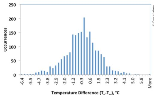
Histogram of asphalt pavement subsurface temperature difference (predicted ( $T_p$ )-measured ( $T_m$ ) temperature difference). © Dong Wang
