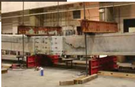
Full-scale flexural test of a beam splice connection made of UHPC.
