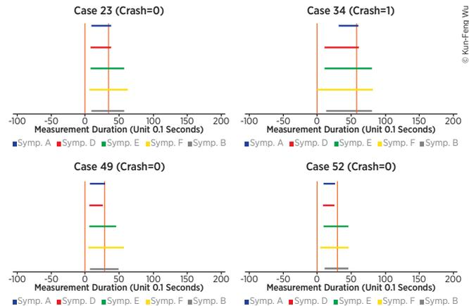
The crash symptoms (horizontal lines) as they compare to manual identification of a crash-related event (vertical red lines). This exhibits the potential of surrogate measures to predict safety-related events based on kinematic and environmental factors.
