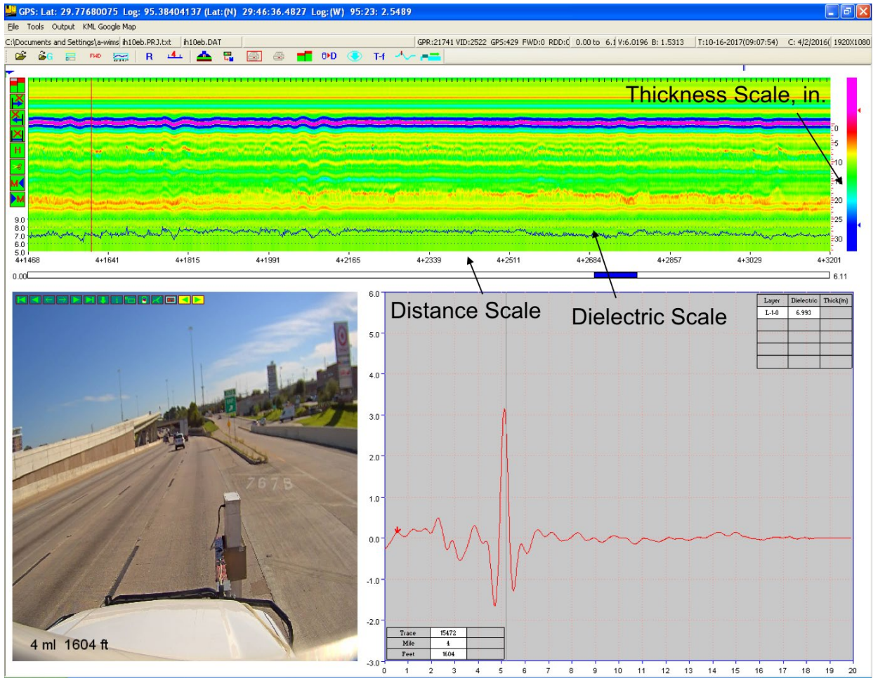
Figure 32. GPR Data Analysis on a Section of I-10.
