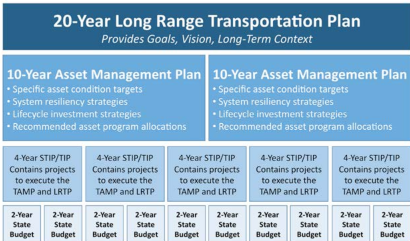
Figure 1. The relationship between long-range plans, asset management plans, TIPs and State budgets.
